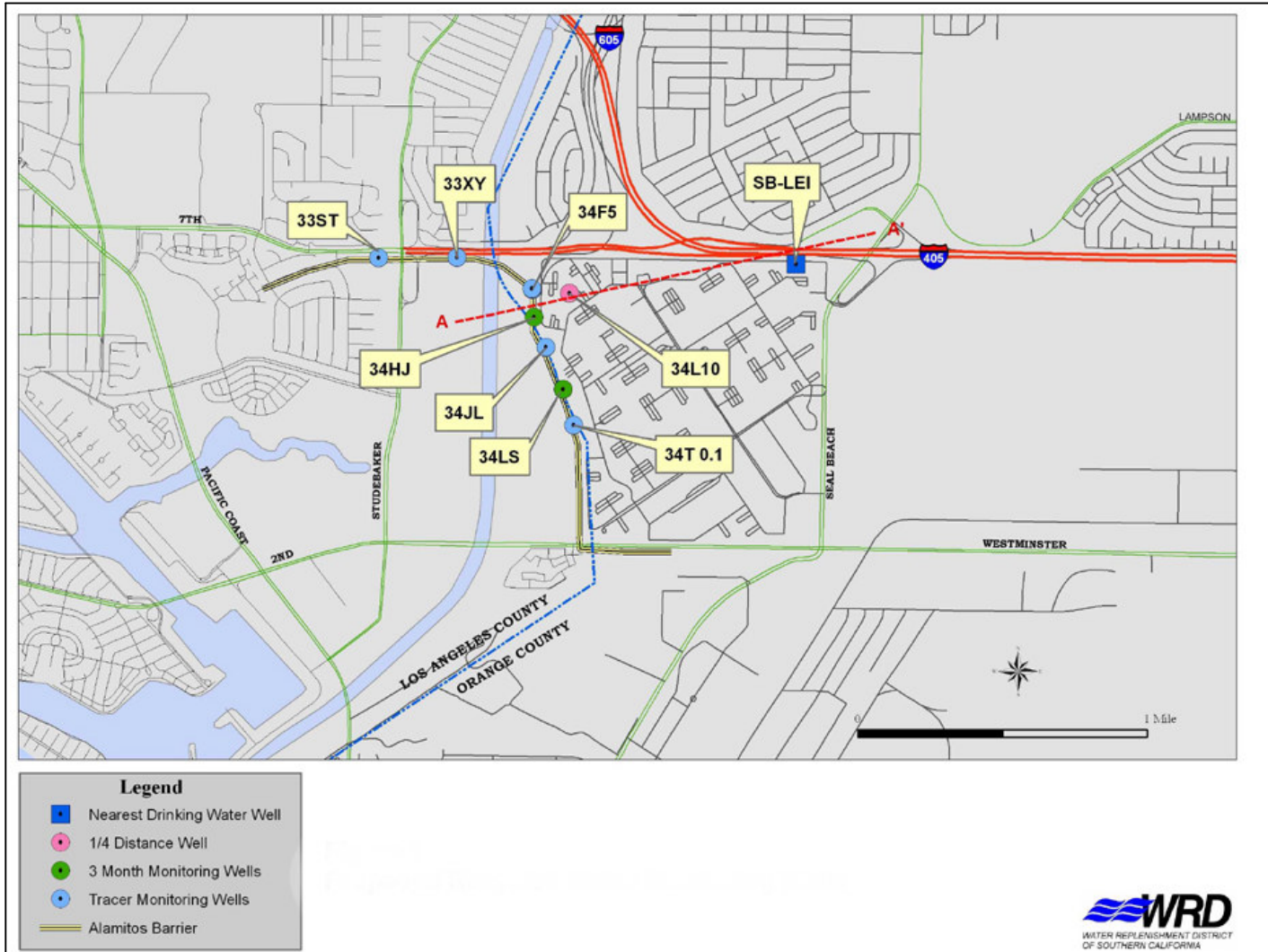
Figure P7- Groundwater Monitoring Well Locations of Alamitos Barrier Recycled Water Project
