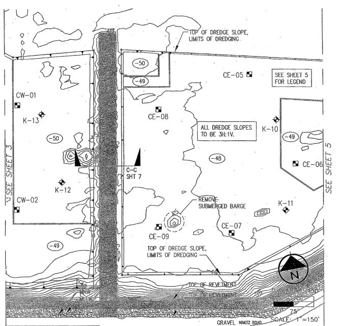
Figure 5. Dredging plan for AOEC-C East and West for IR Site 7.
