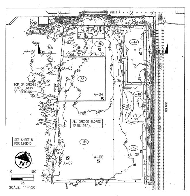
Figure 3. Dredging plan for AOEC-A for IR Site 7.
