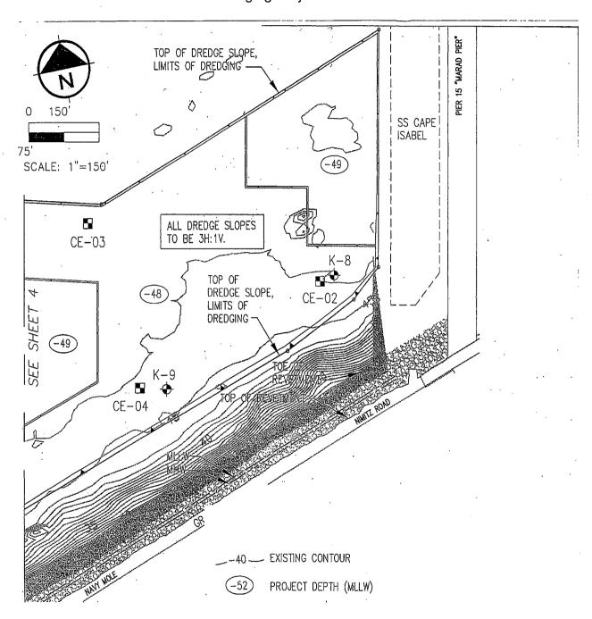
Figure 6. Dredging plan for AOEC-C West for IR Site 7.
