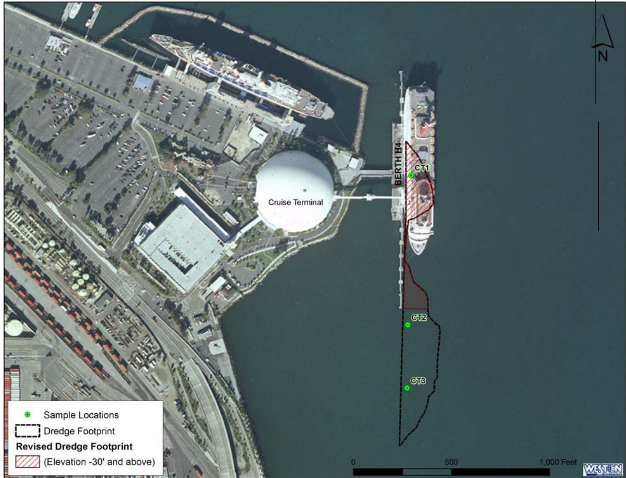
Figure 2. Areas to be dredged for Carnival Passenger Terminal Berth Maintenance Dredging in Long Beach Harbor.
