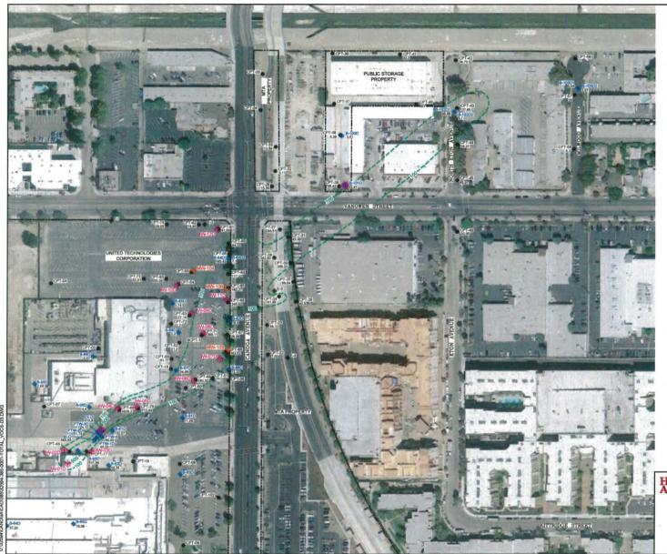
LEGEND: APPROXIMATE PROPERTY LINE MONITORING WELL LOCATION U - UPPER SAND ZONE I - INTERMEDIATE SAND ZONE D - DEEP SAND ZONE FORMER EXTRACTION WELL LOCATION CONE PENETROMETER TEST (CPT) WITH GROUNDWATER GRAB SAMPLES (2006 THROUGH 2014) PROPOSED INJECTION WELL LOCATION EXISTING MONITORING WELL PROPOSED FOR INJECTION PROPOSED MONITORING WELL LOCATION
