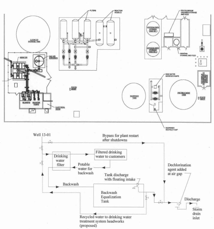
Figure 2. Treatment Schematic
