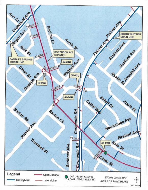
Figure 2. Storm drain map (Discharge Points M-001 - M-005)
