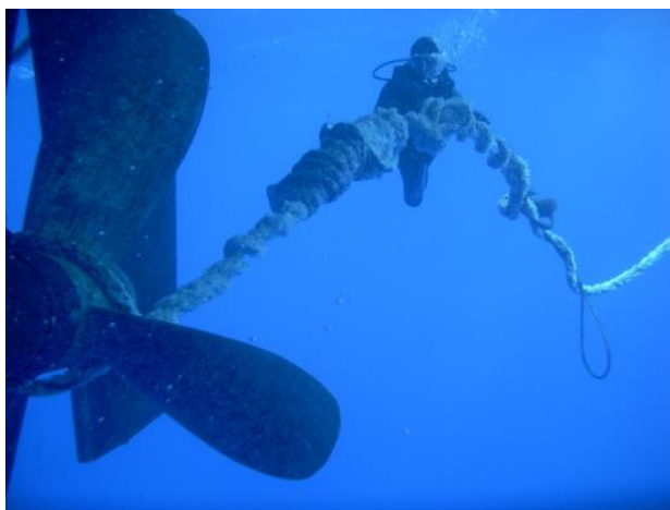
Figure 4. Entangled Propeller (NOAA Marine Debris Program).
