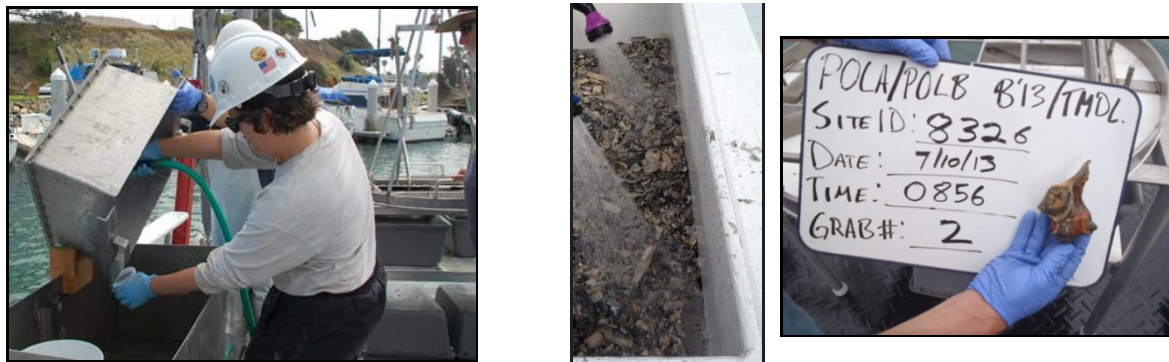
Figure 2-2. Benthic Infaunal Community Collections – Sieving Sediments and Capture of Organisms in the Field for Subsequent Identification
