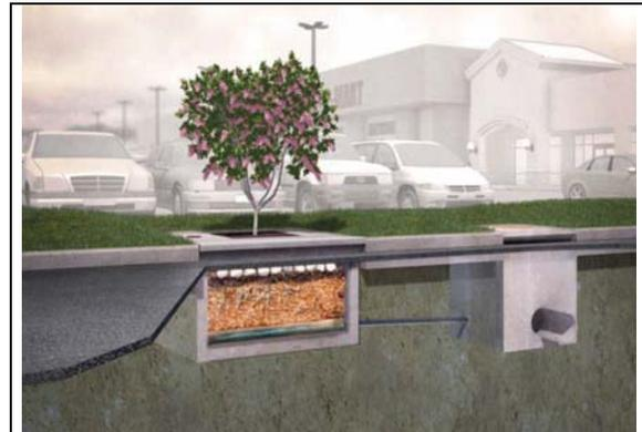
Figure 5-5. Bacteria™ Bioretention Technology
