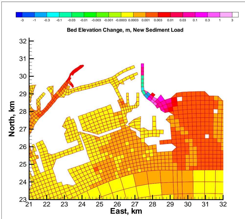
Figure 2. Bed elevation change using hourly flow and sediment loads from the Los Angeles River
