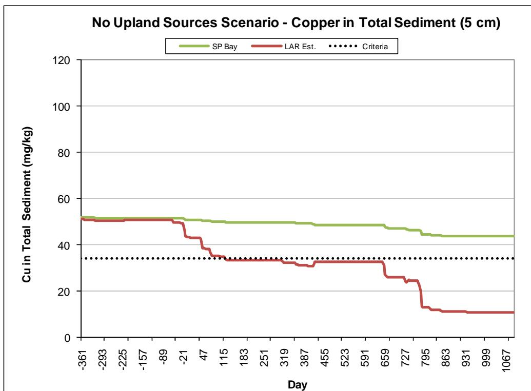
Figure 7. Sediment copper concentrations for the no upland sources scenario
