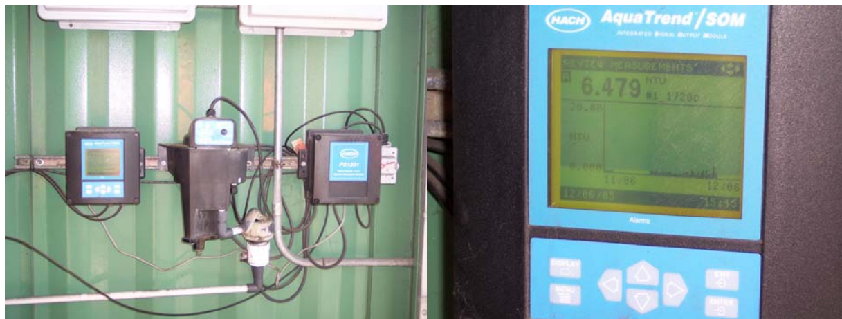
Figures 3.1 and 3.2 Hach 1720D Nephelometer used to analyze turbidity in influent water.
