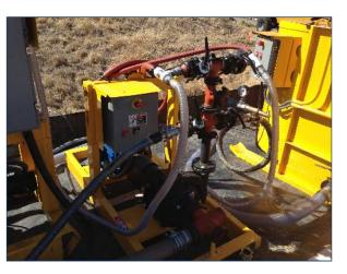
Figure 2 – Sheer pump used to create a uniform guar mixture to adequately suspend ZVI
