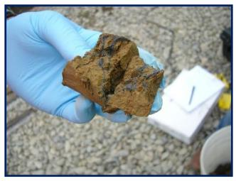
Figure 2 – DPT Core Showing ZVI Throughout Core
