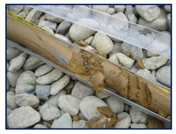
Figure 1 – DPT Core Showing ZVI Distribution 10 to 11 feet bgs
