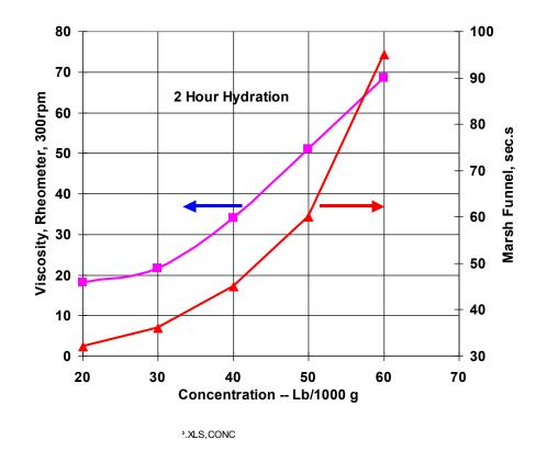
Figure 1: Viscosity with Concentration shows fresh water viscosity for a range of concentrations of Rantec G150 biopolymer.
