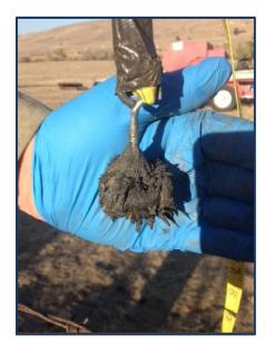
Figure 1 – Magnet recovering ZVI from target monitoring well 15' from injection location
