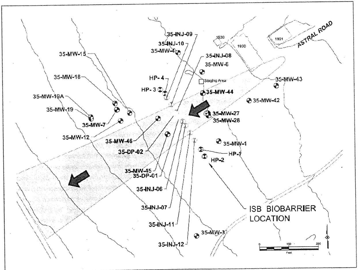
**Exhibit 1.** The arrows indicate the approximate direction of groundwater flow and TCE plume migration. The plume contour represents the approximate 50 micrograms per liter TCE in groundwater prior to the biobarrier installation
