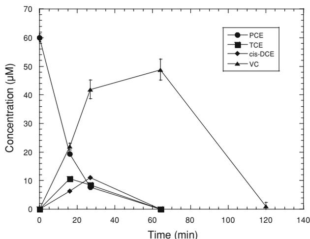
**Fig. 4** Results of a PCE degradation assay with samples from a 550-L fermentation batch of the SDC-9<sup>TM</sup> culture. The assay was performed in 60-mL serum vials containing 60 mL SDC-9<sup>TM</sup> culture (0.52 g/L Dwt), 6 mM sodium lactate, and 10 mg/L PCE. Values represent means of triplicate samples and error bars represent one standard error of the mean
