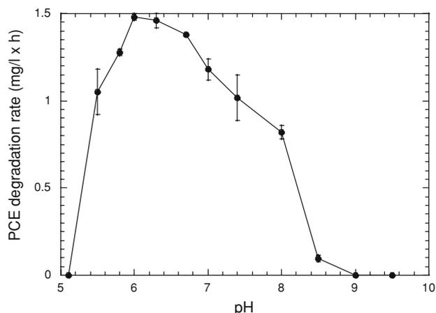
**Fig. 3** Effect of culture pH on PCE dehalogenation by SDC-9™. Values represent the mean of triplicate samples, and *error bars* represent one standard error of the mean
