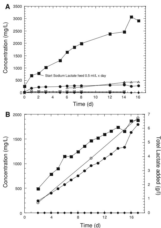
**Fig. 2** Accumulation of VFAs during growth of SDC-9<sup>TM</sup> (a) or PJKS<sup>TM</sup> (b) in a 750-L fermentor. Symbols indicate lactic acid (filled diamond), propionic acid (filled circle), formic acid (open diamond), pyruvic acid (open square), butyric acid (open triangle), and acetic acid (filled square), or the total amount of sodium lactate added to the fermentor (open circle; b)
