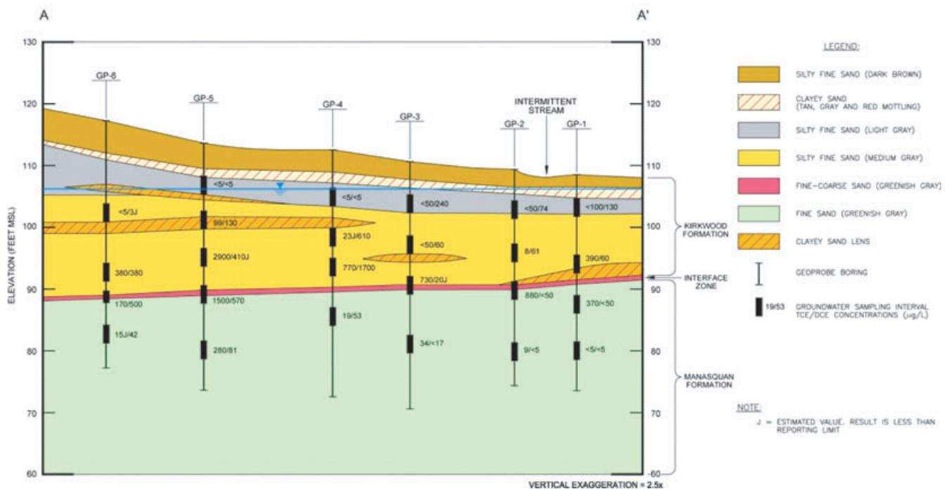
Figure 1. Demonstration area's geologic cross section and contaminant distribution.
