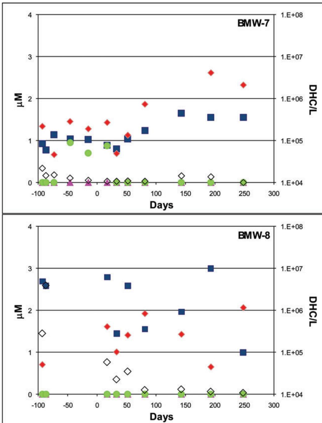
**Figure 6. Ethenes and DHC concentrations plotted as a function of time for loop 4 (control loop). Bioaugmentation was performed at 0 days.  $\diamond$ , TCE;  $\blacksquare$ , DCE;  $\blacktriangle$ , vinyl chloride;  $\bullet$ , ethene;  $\blacklozenge$ , DHC. No detection of vinyl chloride or ethene were observed.**
