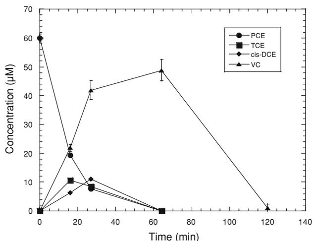
**Fig. 4** Results of a PCE degradation assay with samples from a 550-L fermentation batch of the SDC-9™ culture. The assay was performed in 60-mL serum vials containing 60 mL SDC-9™ culture (0.52 g/L Dwt), 6 mM sodium lactate, and 10 mg/L PCE. Values represent means of triplicate samples and *error bars* represent one standard error of the mean
