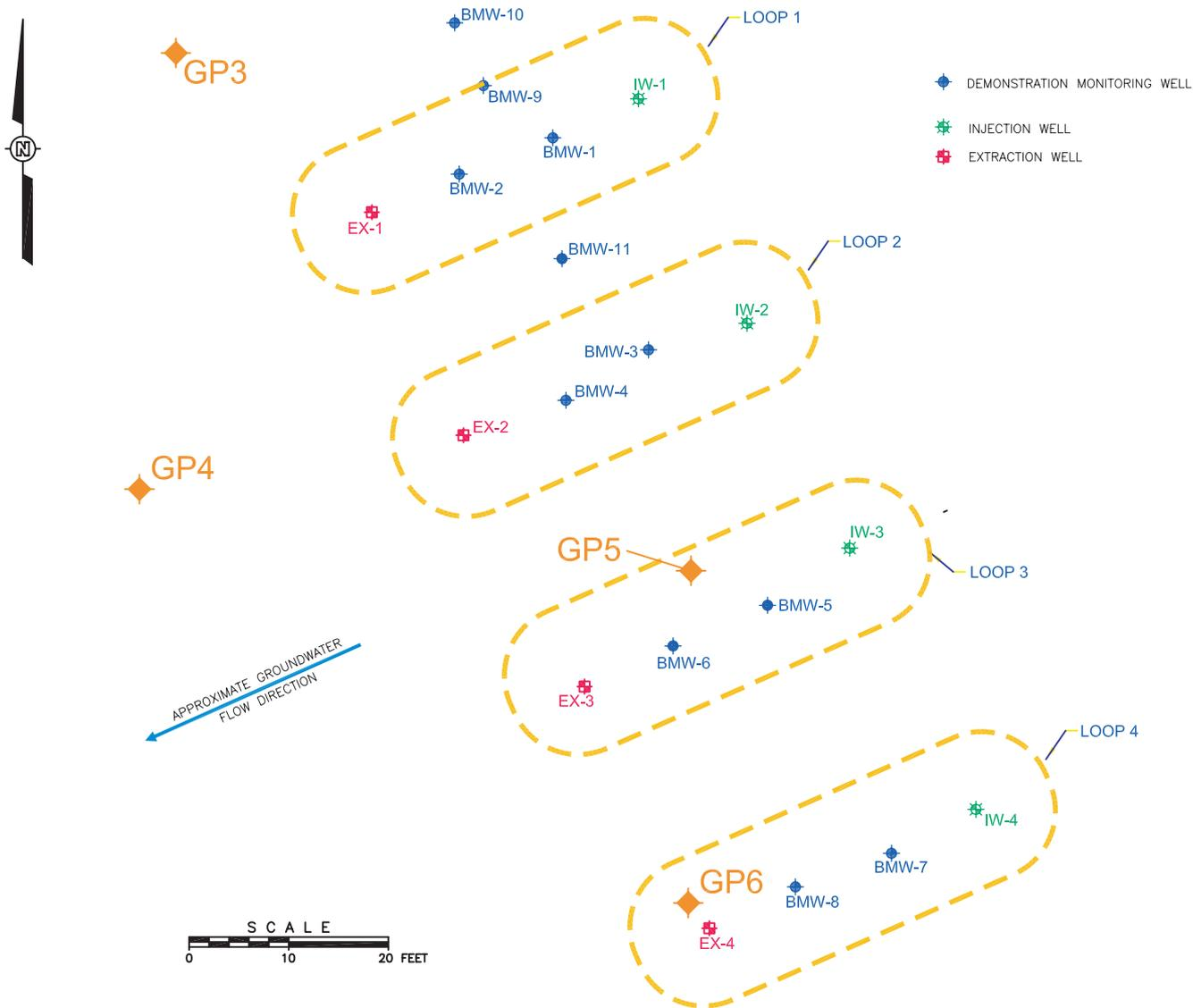
**Figure 2. Demonstration layout.**
