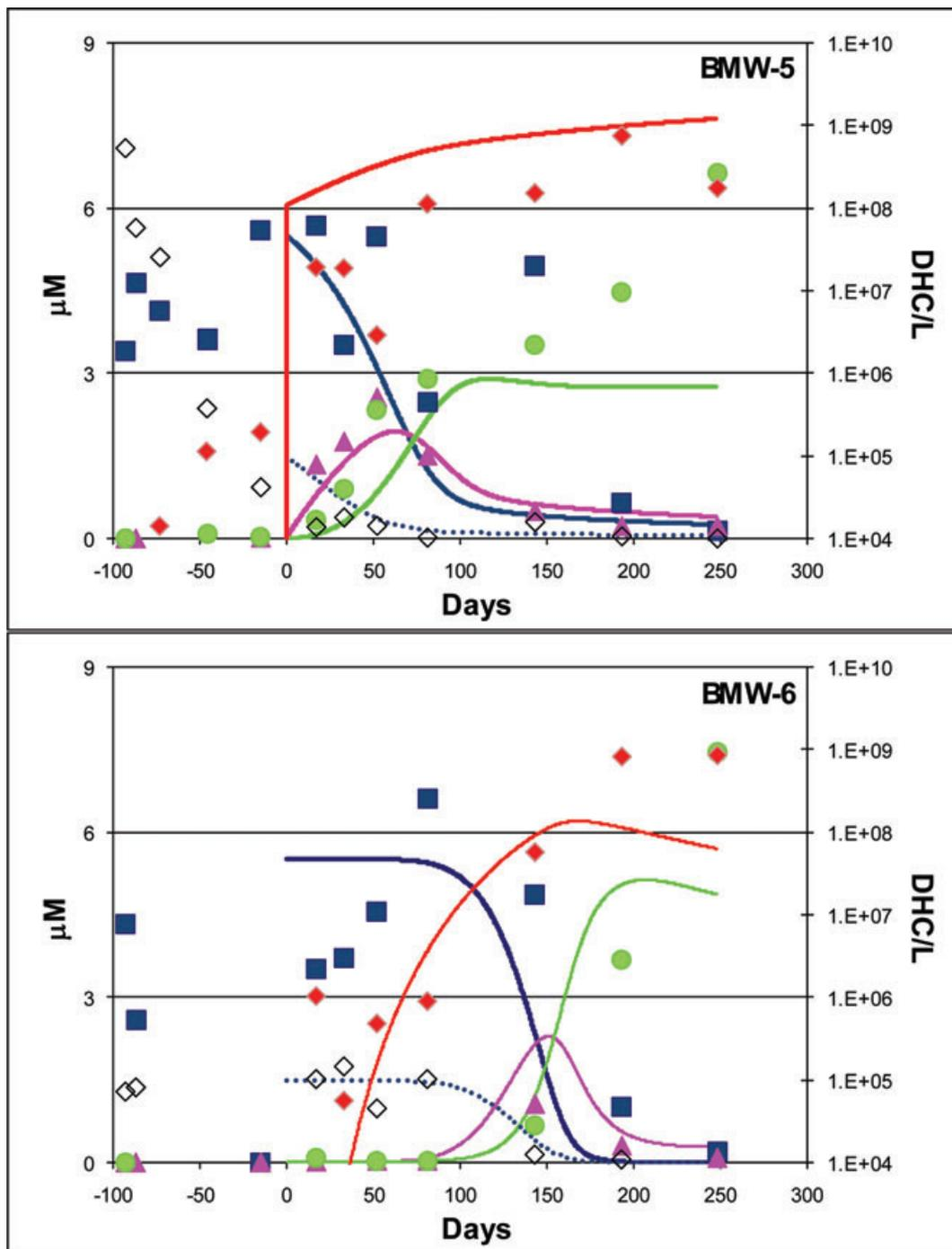
Figure 5. Ethenes and DHC concentrations plotted as a function of time for loop 3. Bioaugmentation was performed at 0 days.  $\diamond$ , TCE;  $\blacksquare$ , DCE;  $\blacktriangle$ , vinyl chloride;  $\bullet$ , ethene;  $\blacklozenge$ , DHC. Solid and dotted lines represent corresponding model simulations. Simulated DHC concentrations in the bioaugmentation injection well (BMW-5) include the total (mobile and immobile) DHC.
