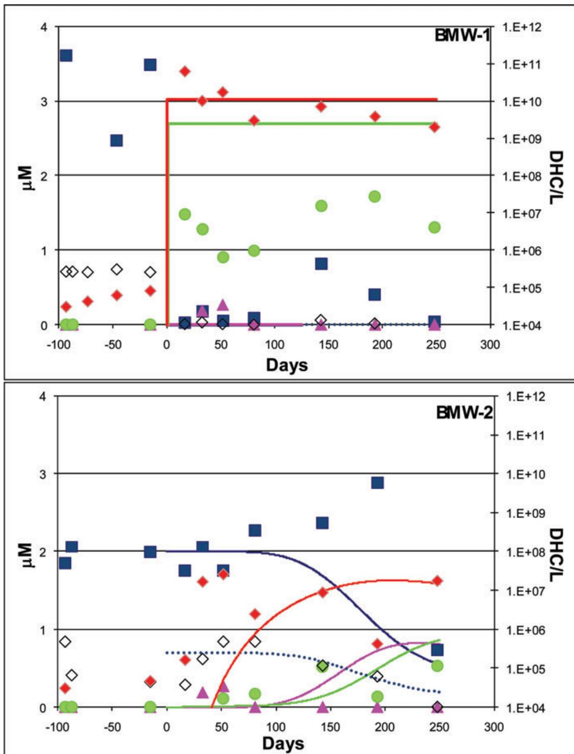
Figure 3. Ethenes and DHC concentrations plotted as a function of time for loop 1. Bioaugmentation was performed at 0 days.  $\diamond$ , TCE;  $\blacksquare$ , DCE;  $\blacktriangle$ , vinyl chloride;  $\bullet$ , ethene;  $\blacklozenge$ , DHC. Solid and dotted lines represent corresponding model simulations. Simulated DHC concentrations in the bioaugmentation injection well (BMW-1) include the total (mobile and immobile) DHC.
