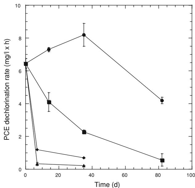
**Fig. 5** Effect of storage conditions on the activity of concentrated SDC-9<sup>TM</sup> culture. Tenfold-concentrated SDC-9<sup>TM</sup> culture was stored anaerobically and without substrate at either 4°C (filled circle), 13°C (filled square), 22°C (filled diamond) or 28°C (filled triangle). Values represent means of triplicate samples, and error bars are one standard error of the mean
