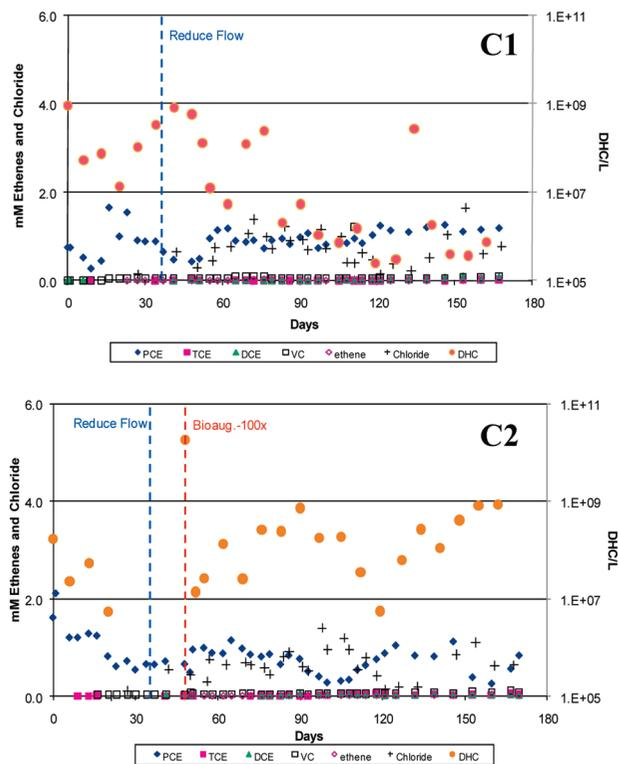
**FIGURE 3.** Effluent concentrations of ethenes, chloride, and DHC from rock C1 (top) and C2 (bottom) in Experiments 5 and 6, respectively. Fractures were bioaugmented on Day 0. The vertical lines indicate when the fractures flow was decreased or when inoculation with additional culture was performed.
