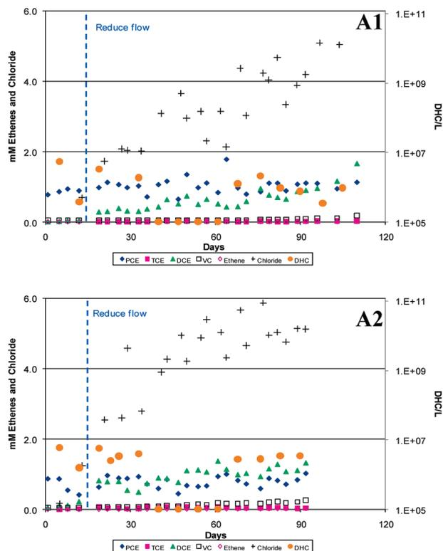
**FIGURE 2.** Effluent concentrations of ethenes, chloride, and DHC from rock A1 (top) and A2 (bottom) in Experiments 3 and 4, respectively. Fractures were bioaugmented on Day 0. The vertical lines indicate when the fractures flow was decreased from approximately 0.10 cm<sup>3</sup>/min to 0.025 cm<sup>3</sup>/min. Experiment 4 was terminated prior to Experiment 3.
