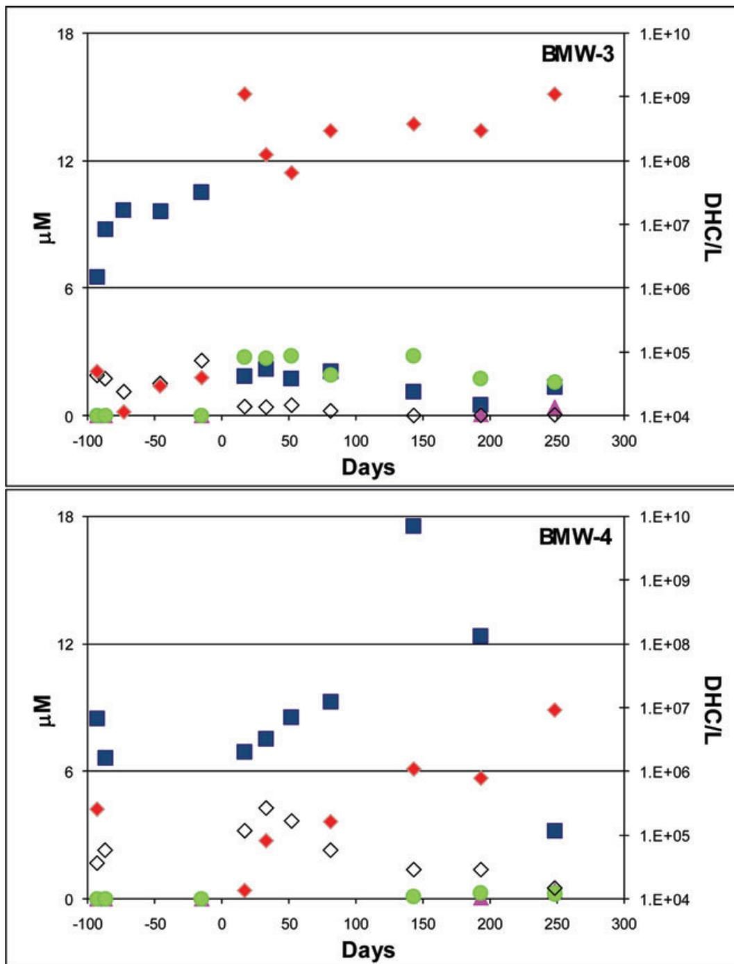
Figure 4. Ethenes and DHC concentrations plotted as a function of time for loop 2. Bioaugmentation was performed at 0 days.  $\diamond$ , TCE;  $\blacksquare$ , DCE;  $\blacktriangle$ , vinyl chloride;  $\bullet$ , ethene;  $\blacklozenge$ , DHC.
