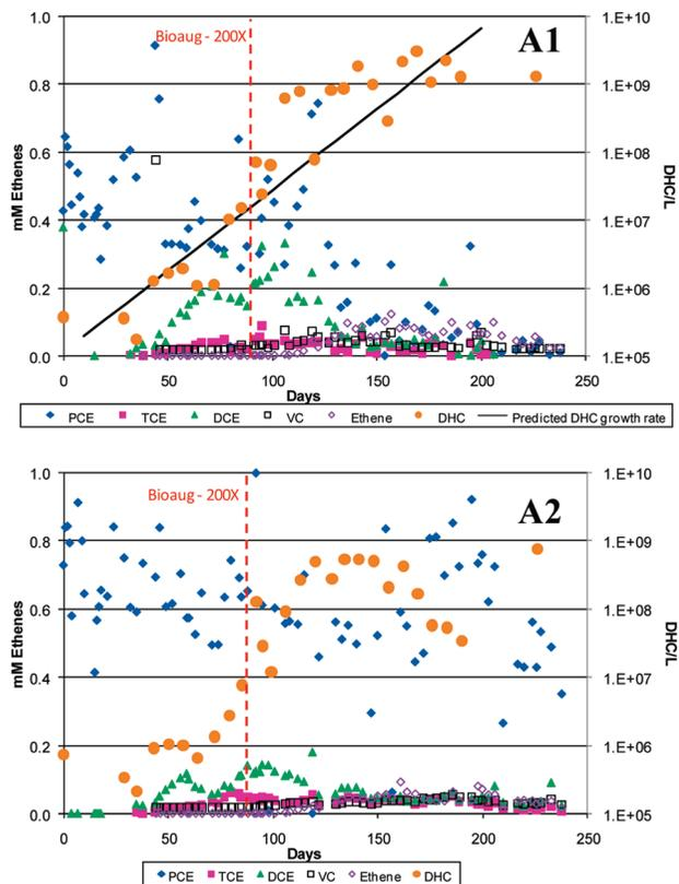
**FIGURE 1. Effluent concentrations of ethenes and DHC from rock A1 (top) and A2 (bottom) in Experiments 1 and 2, respectively. Fractures were bioaugmented on Day 0. The vertical dashed lines indicate when inoculation with additional culture was performed. The solid line for A1 represents the predicted rate of DHC growth (5). For A2, some interruptions in flow occurred between days 150 and 190. Chloride concentrations were not monitored in Experiments 1 and 2.**
