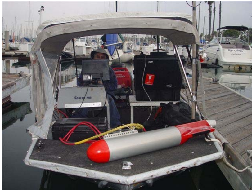
Photograph 2. Imagenex 881 Sportscan Side Scan Sonar
