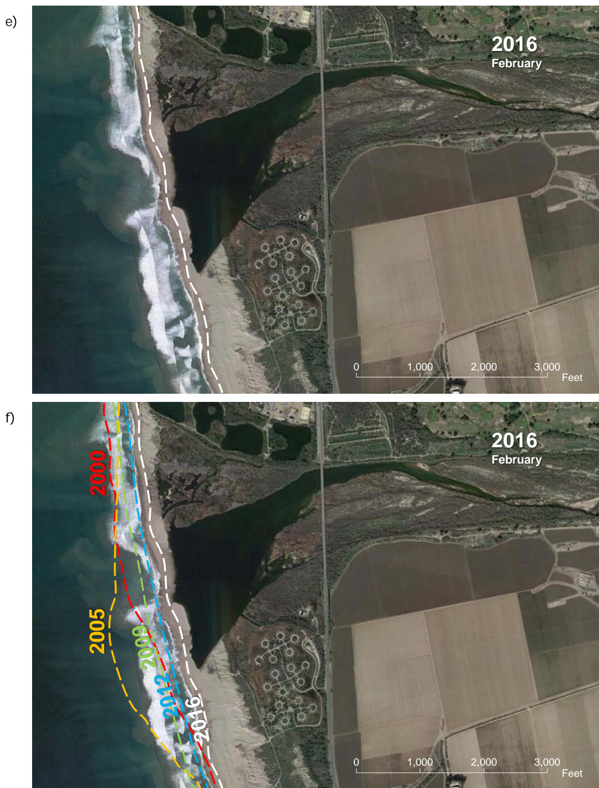
Figure C-8. Repeat aerial photographic views of the SCRE during 2000 (a), 2005 (b), 2009 (c), 2012 (d), and 2016 (e), with combined overlay of beach berm positions (f). Imagery sources from State Parks and NAIP.
