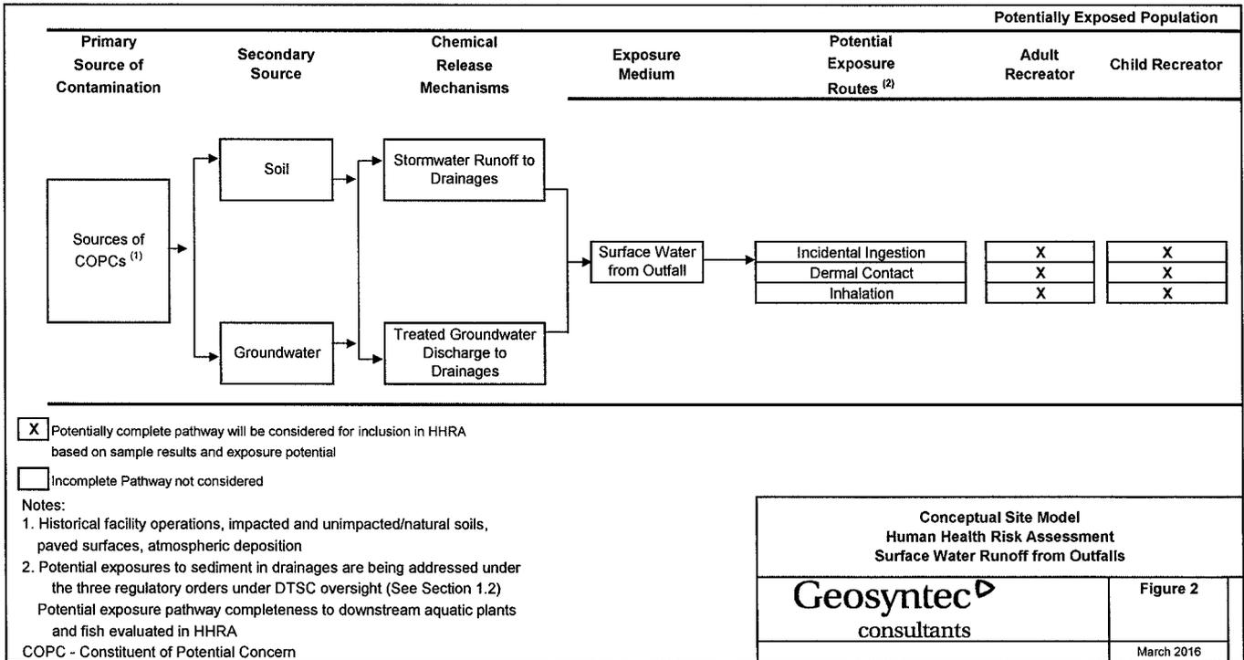
Figure 2 - HHRA CSM\_SSFL SW Runoff HHRA
