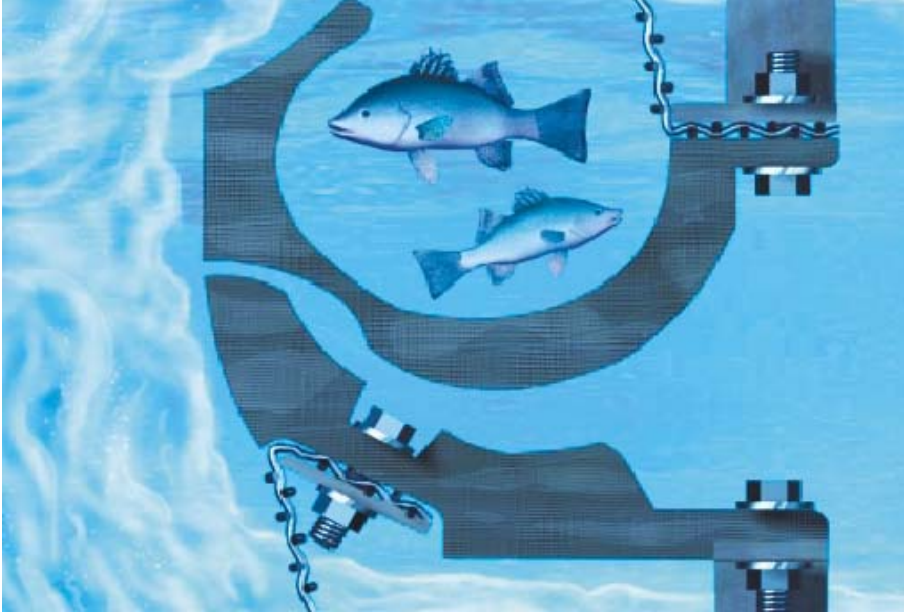
Figure 9 Ristroph screen buckets attached to bottom of traveling screen panels.
