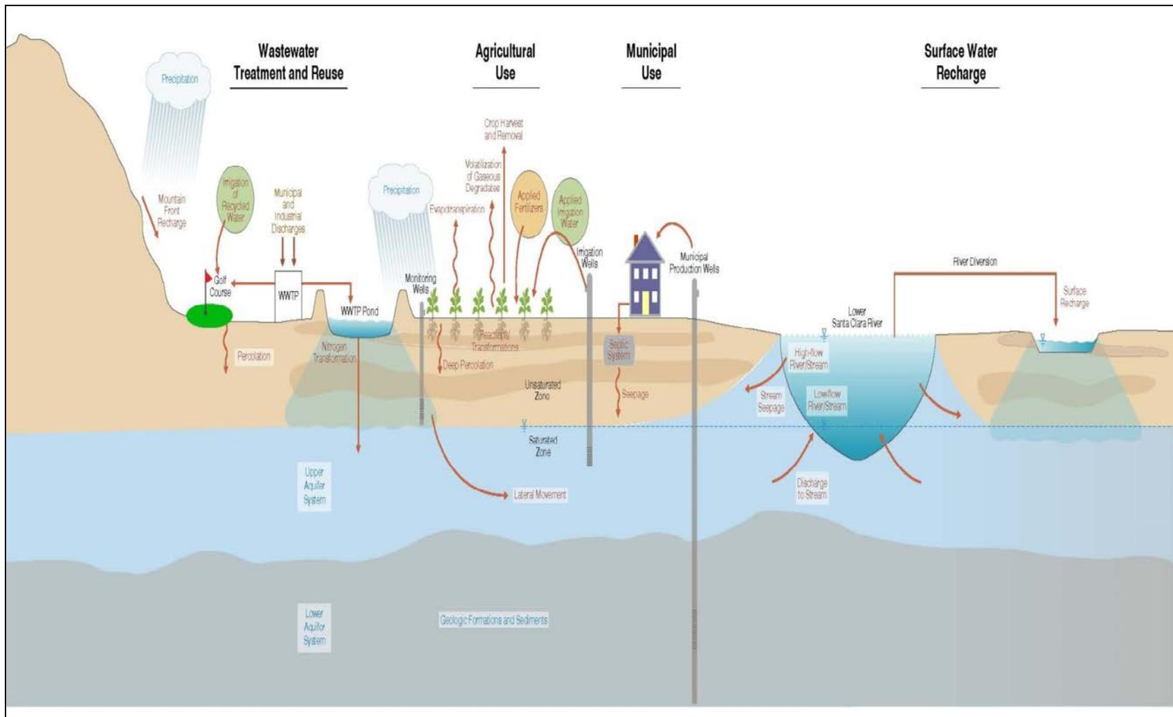
**Figure 6-1 Conceptual Model of Salt and Nutrient Contributions**
