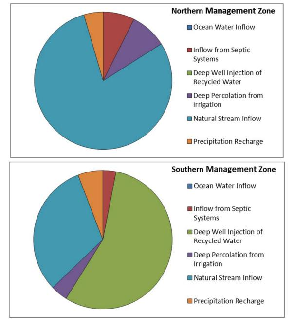
Figure 4-18: Inflows to Malibu Valley Groundwater Basin by Component – Phase 2 of CCWTF Project
