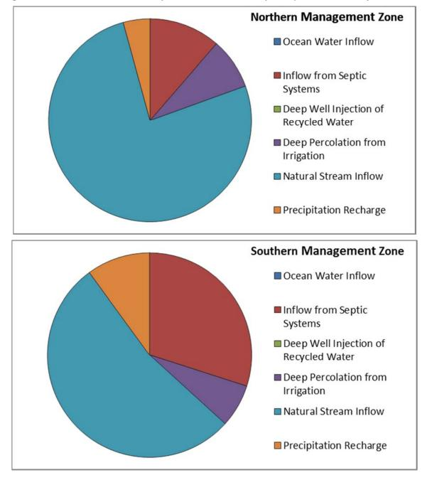
Figure 4-16: Inflows to Malibu Valley Groundwater Basin by Component - No Project Scenario
