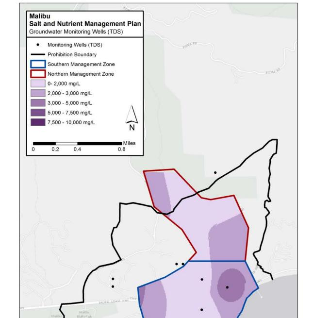
Figure 4-3: Total Dissolved Solids Concentrations in the Malibu Valley Groundwater Basin
