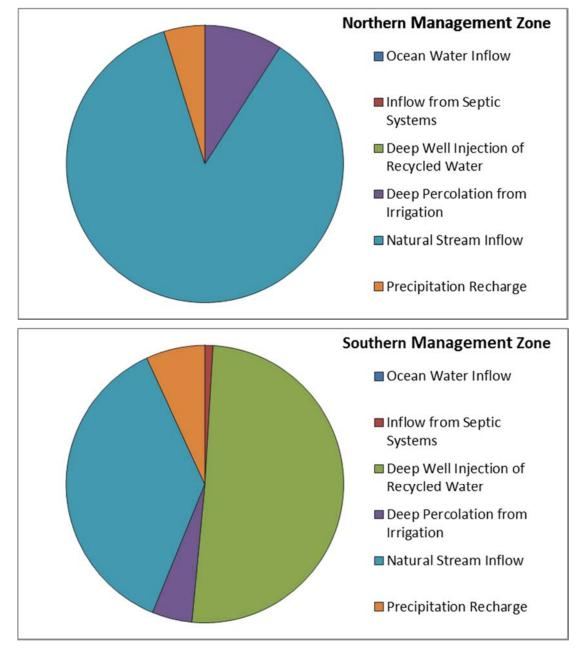
Figure 4-19: Inflows to Malibu Valley Groundwater Basin by Component – Phase 3 of CCWTF Project
