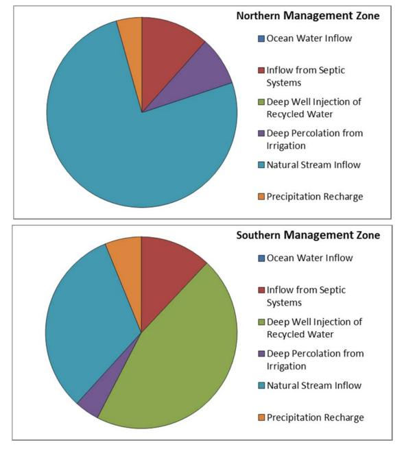
Figure 4-17: Inflows to Malibu Valley Groundwater Basin by Component – Phase 1 of CCWTF Project
