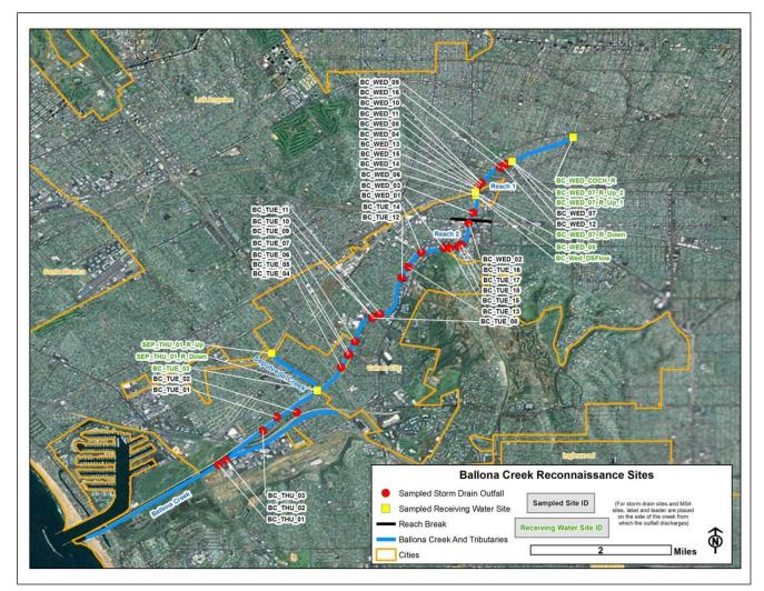
Figure 3. Storm Drain Outfalls and Receiving Water Sites Sampled During June 2012 Ballona Creek Reconnaissance Study
