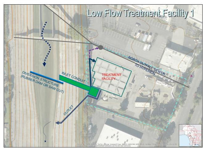
Figure 7. Plan View of the LFTF #1
