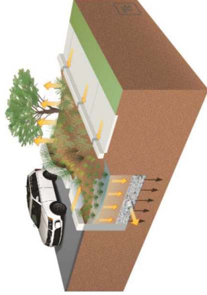
Typical distributed bioretention and biofiltration schematic showing underdrain option (arrows indicate water pathways).
