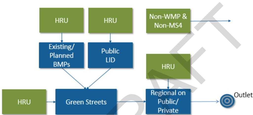
Figure A-1. Conceptual schematic illustrating BMP routing for the RAA
