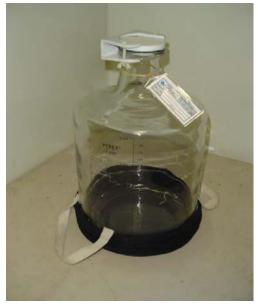
Figure 2. Composite bottle showing bottle bag used for transport and lifting.
