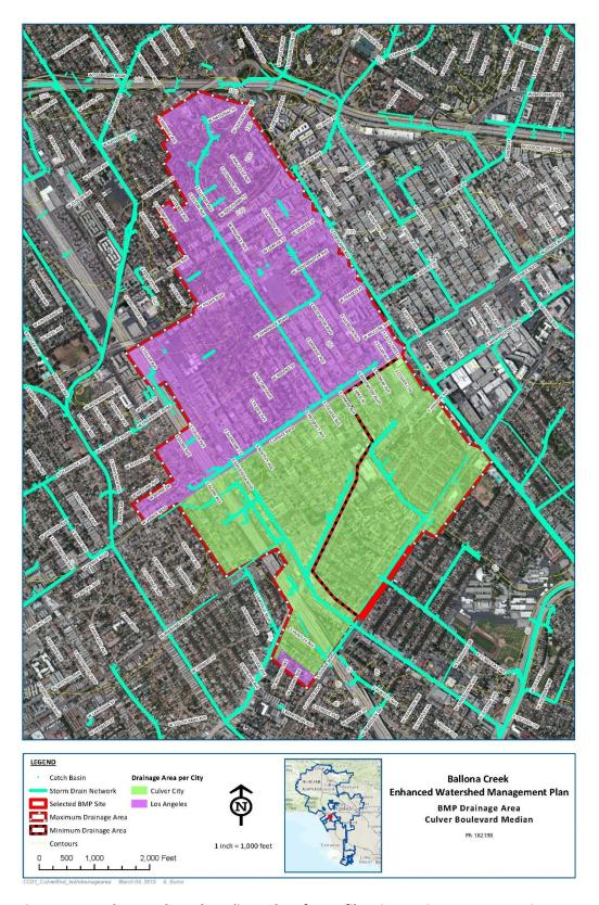
Figure 4-14 Culver Boulevard Median Subsurface Infiltration Drainage Area – Drainage Map
