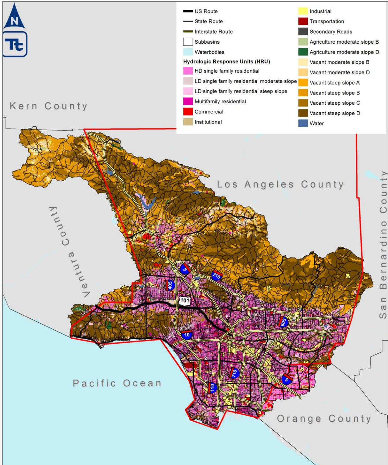
Figure 4-1 WMMS Model Domain, Representative Land Uses, and Slopes by Subwatershed
