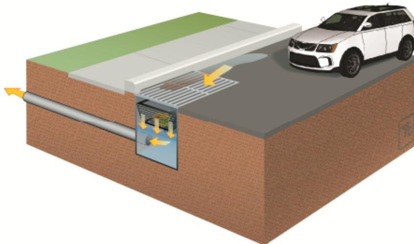
Typical distributed source control structural BMP (arrows indicate water pathways).
