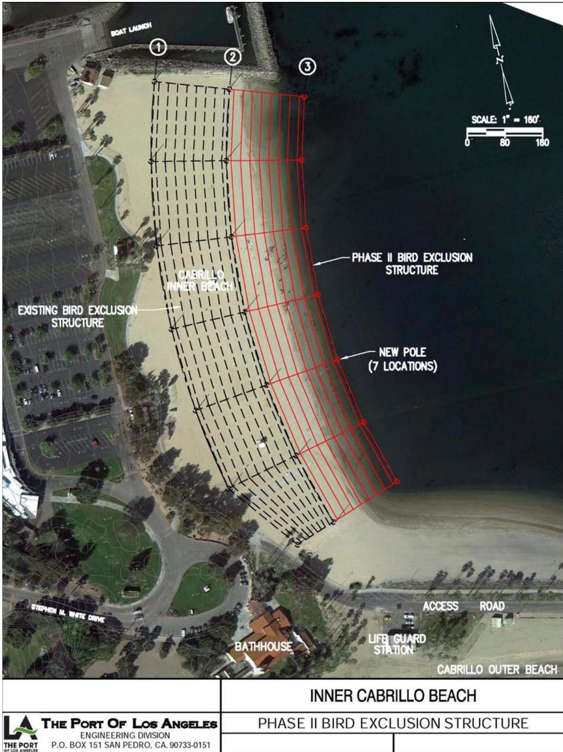
Figure 4. Bird Exclusion Structure (Phase II) Schematic
