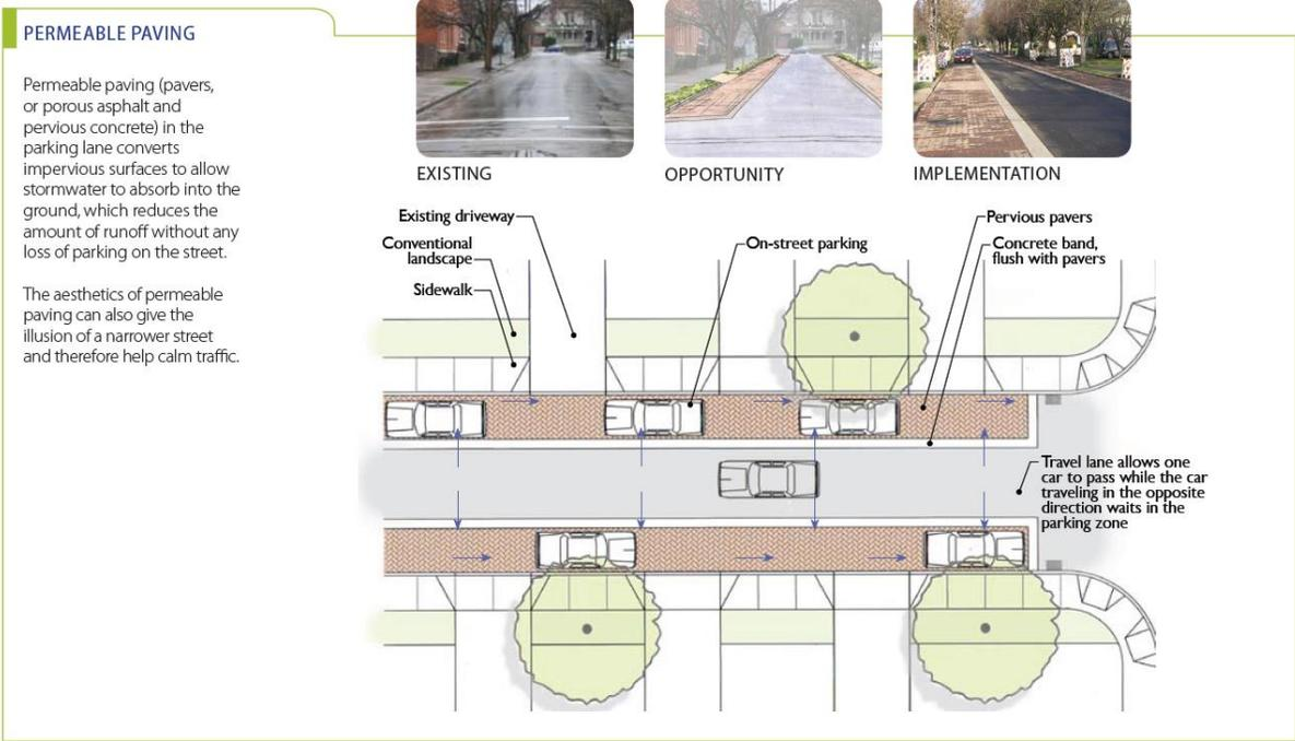
Figure 17: Green Streets with Permeable Pavement (EPA, 2009)
