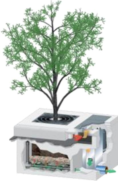
Figure 14: Biofiltration Device
