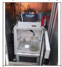
Figure C-1. ISCO Type **Automated Flow and Sampling Equipment Installed at Existing Monitoring Stations**
