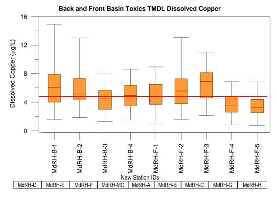
Figure H-1. Marina del Rey Toxics TMDL Dissolved Copper Compliance Monitoring Results (2010-2013)
