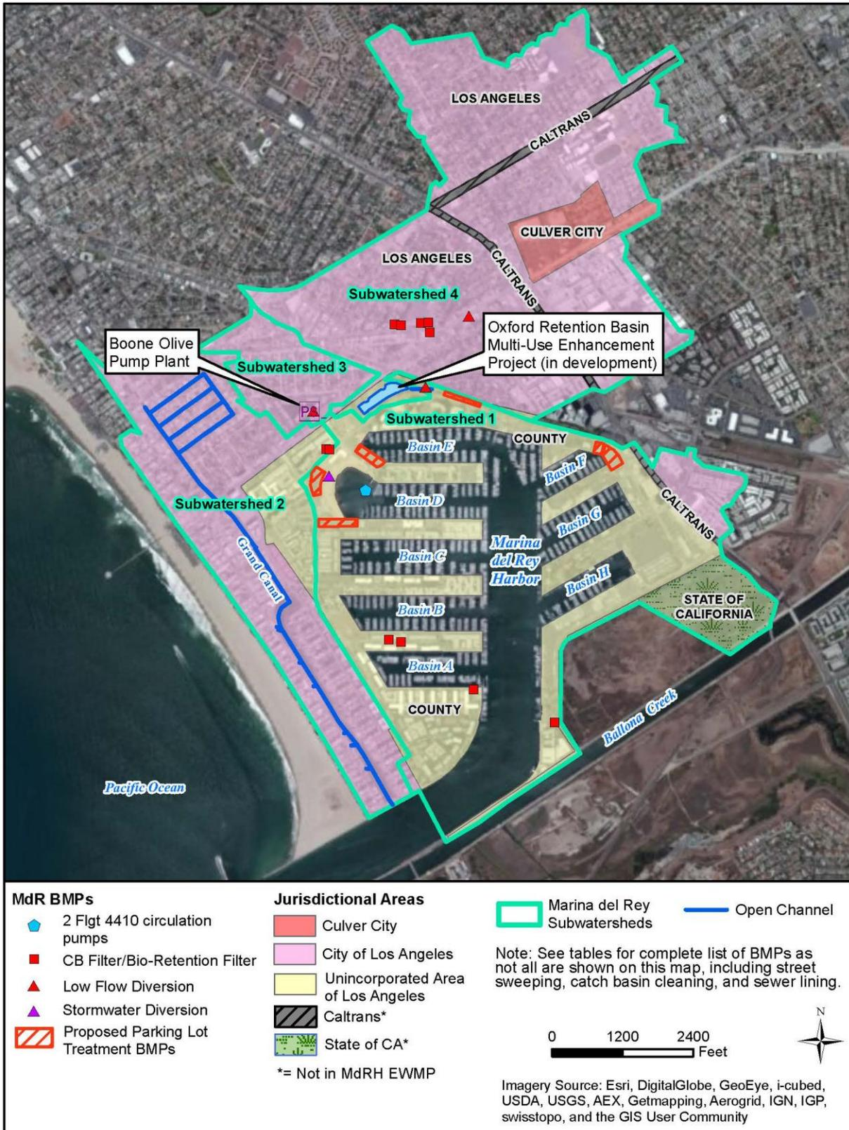
Figure 12. Existing Structural Control Measures within MdrH Boundaries
