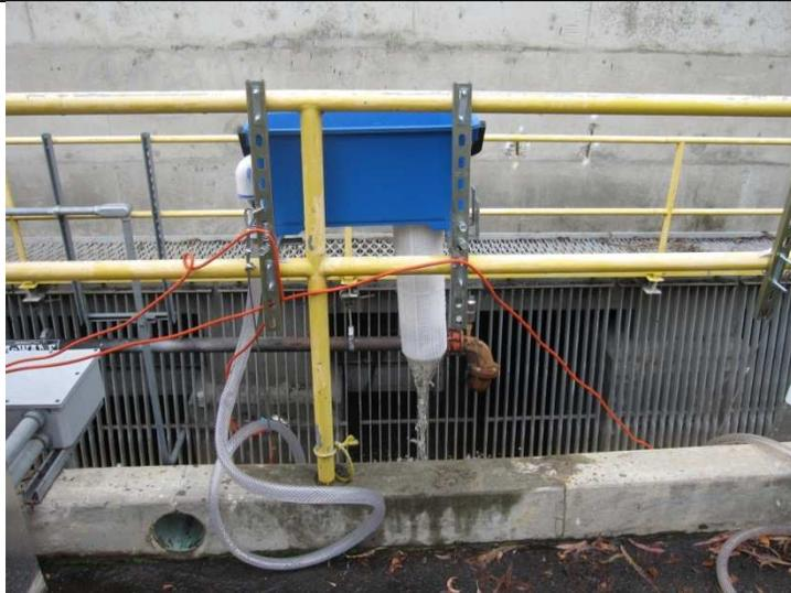
The sample collection system is a bucket with a filter inside. This version is fabricated out of off the shelf components and is attached to a stainless steel pump that is place in the wet well. The pump operates at approximately 5 gpm, depending on the depth of the wet well and the sediment saturation of the filter. Once the pump rate exceeds the filtration rate the excess flow overflows back to the wet well
