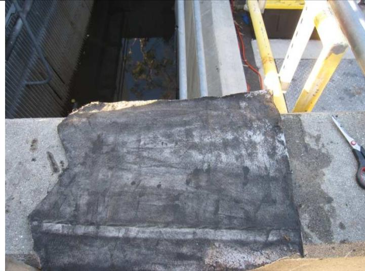
This is what a typical filter that was fully coated with sediments would look like after sediment collection. There is staining on the filter from the smaller particles embedded in the filter.
