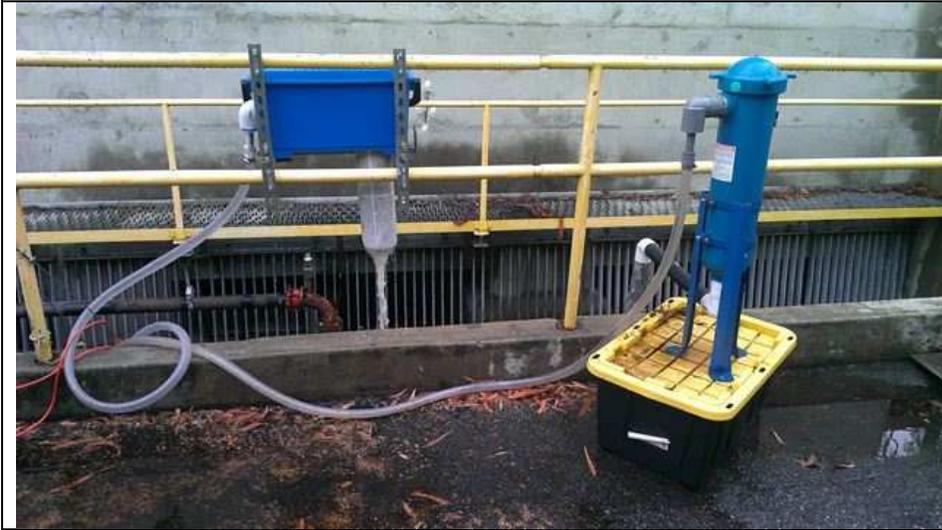
Two different configurations were designed and tested to sample storm-borne sediment from a wet well.
