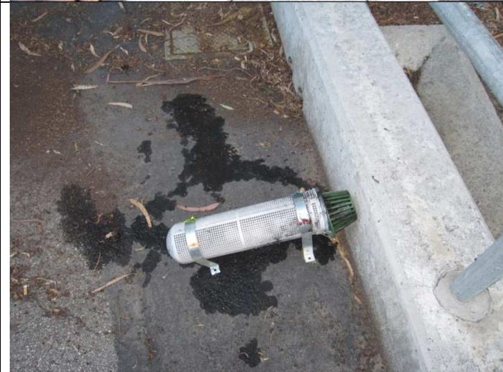
The device typically looks like this upon removal with minimal debris build up on the device.
