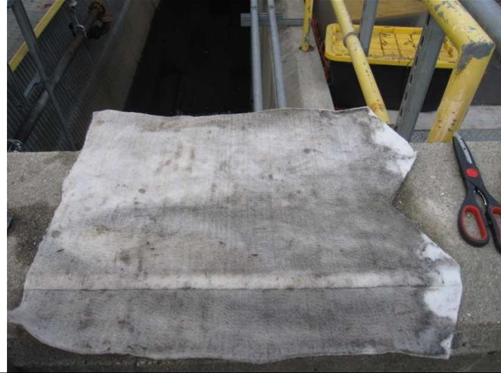
This is a typical filter from a small storm with a low intensity that allowed for the larger particles to settle out limiting the available suspended sediment for collection. Some sediment was collected in the filter to stain the filter; however, there was insufficient sediment to collect a sample.
