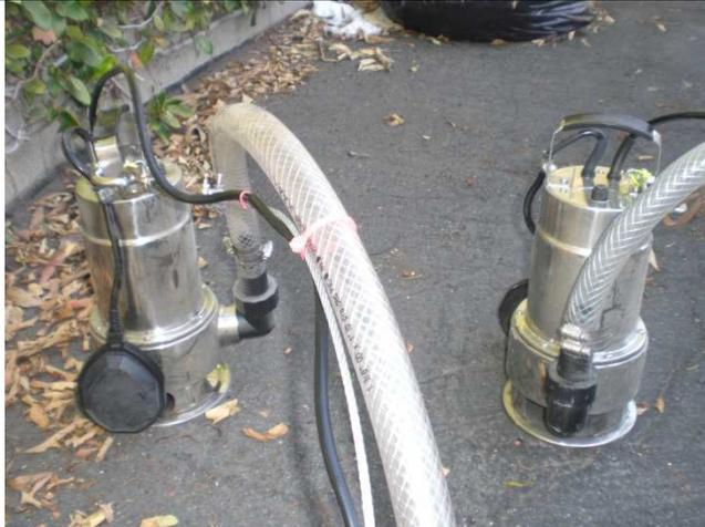
Submersible Pumps were used to sample stormwater from a wet well into each of the devices.
