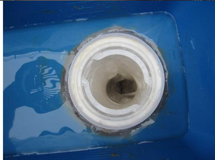
The fresh filter is placed inside the device to allow the water to drain and capture the sediment samples. For the first three events only one filter was used, for the last three events, the filters were replaced once the processing rate and slowed significantly.
