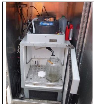
**Figure C-1. ISCO Type Automated Flow and Sampling Equipment Installed at Existing Monitoring Stations**
