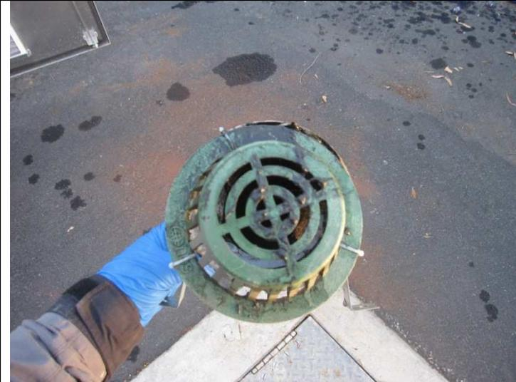
The device typically looks like this upon removal with minimal debris build up on the device. There is evidence of some external sediment build up. For the purposes of the pilot study, this build up was not collected.
