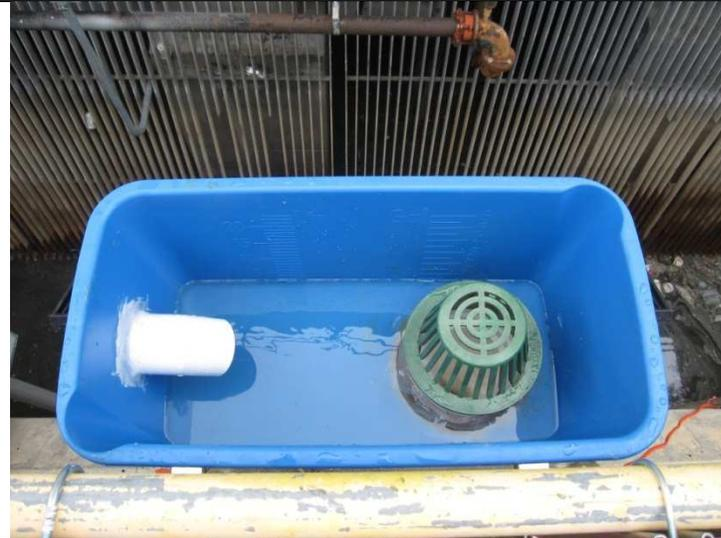
The device is constructed out of a bucket with an inlet and outlet to allow water from the wet well to be pumped up and processed through the filter.
