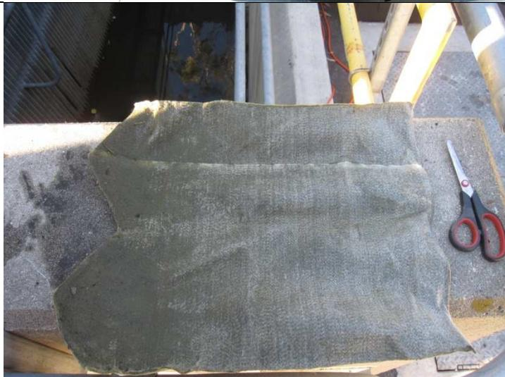
This is a typical filter from a small storm with a low intensity that allowed for the larger particles to settle out limiting the available suspended sediment for collection, however for these events the total solids concentration tended to be low.
