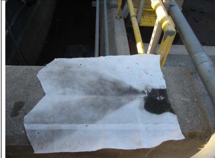
This is a typical filter from a smaller storm in terms of rainfall accumulation and intensity that produces low flow rates within the catch basin and limited opportunity to deposit sediments in the device. Some sediment was collected in the filter to stain the filter; however, there was insufficient sediment to collect a sample.
