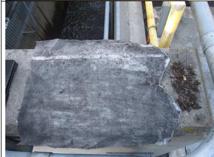
This is what a typical filter that was fully coated with sediments would look like after the loose debris is removed and the sediment is collected. There is staining on the filter from the smaller particles embedded in the filter.
