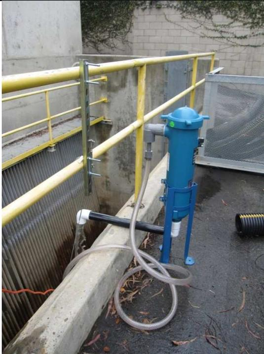
The sample collection system is a pressure cylinder with a filter inside. This version is typically used as a bio-diesel filter that is attached to a stainless steel pump that is placed in the wet well. The pump operates at approximately 5 gpm, depending on the depth of the wet well and the sediment saturation of the filter.
