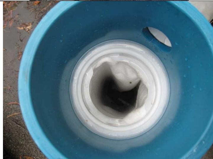
The filter is installed in the top of the device and then sealed inside. The pressure from the pump processes the water through the filter.
