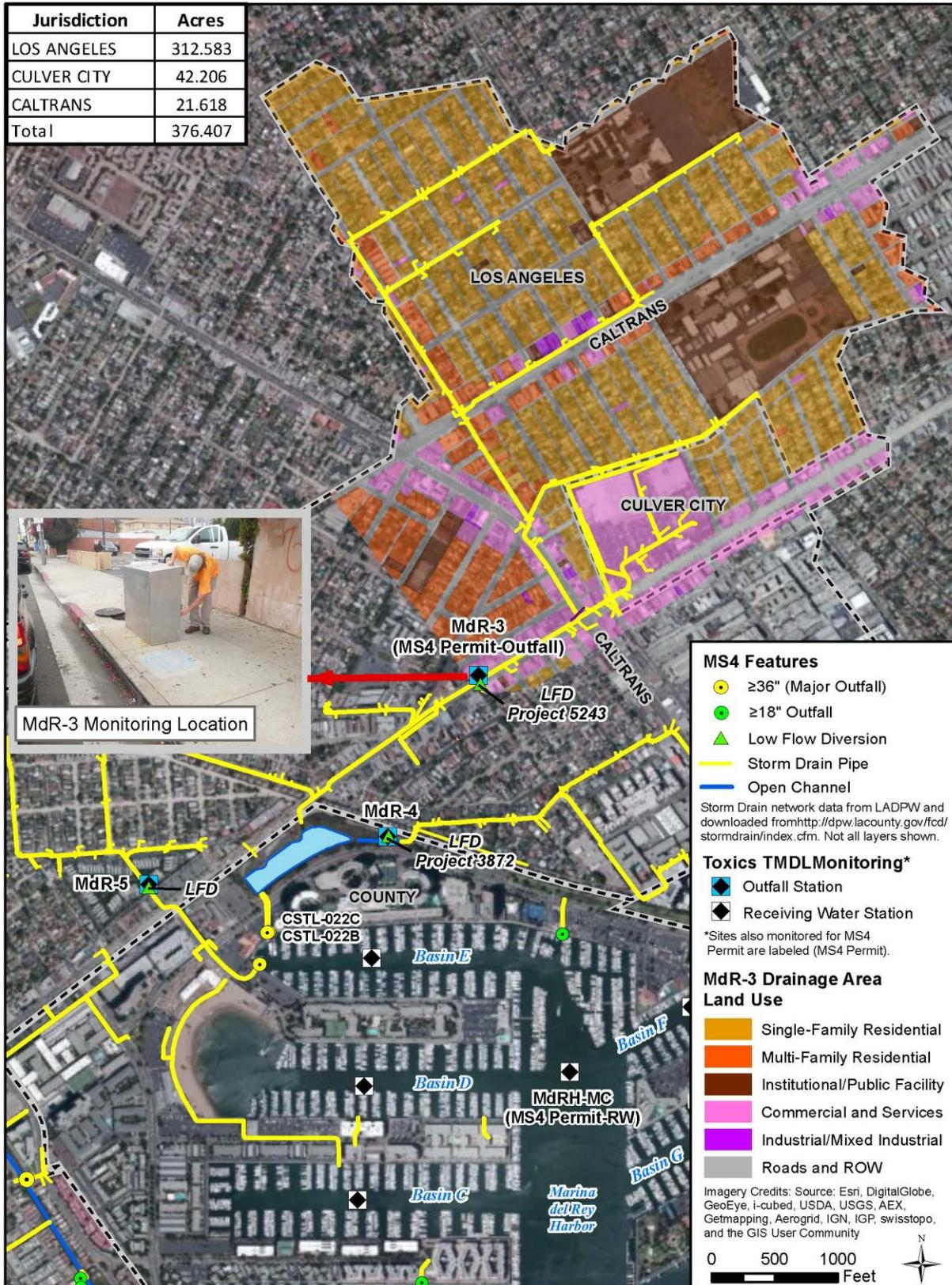
Figure 4-1. Outfall Station Mdr-3 – Permit and Toxics TMDL Monitoring
