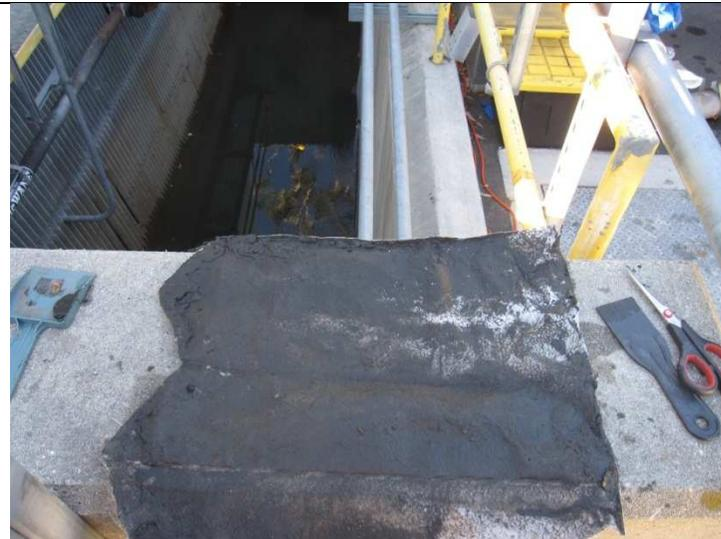
This is a typical filter from a larger storm that produced sufficient intensity to mobilize sediments within the channel instead of settling within the storm drain. The filter is coated in sediment and accumulated small organic debris.
