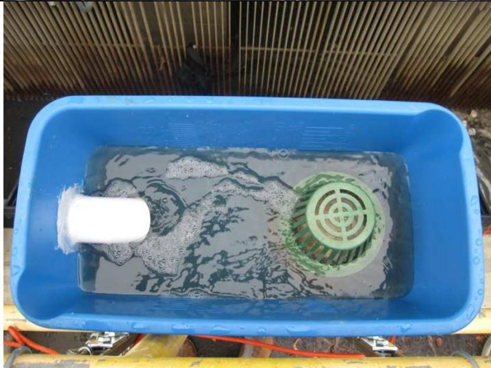
Top view of flow-through device while stormwater from the Boone-Olive Pump Station is processed through the filter.
