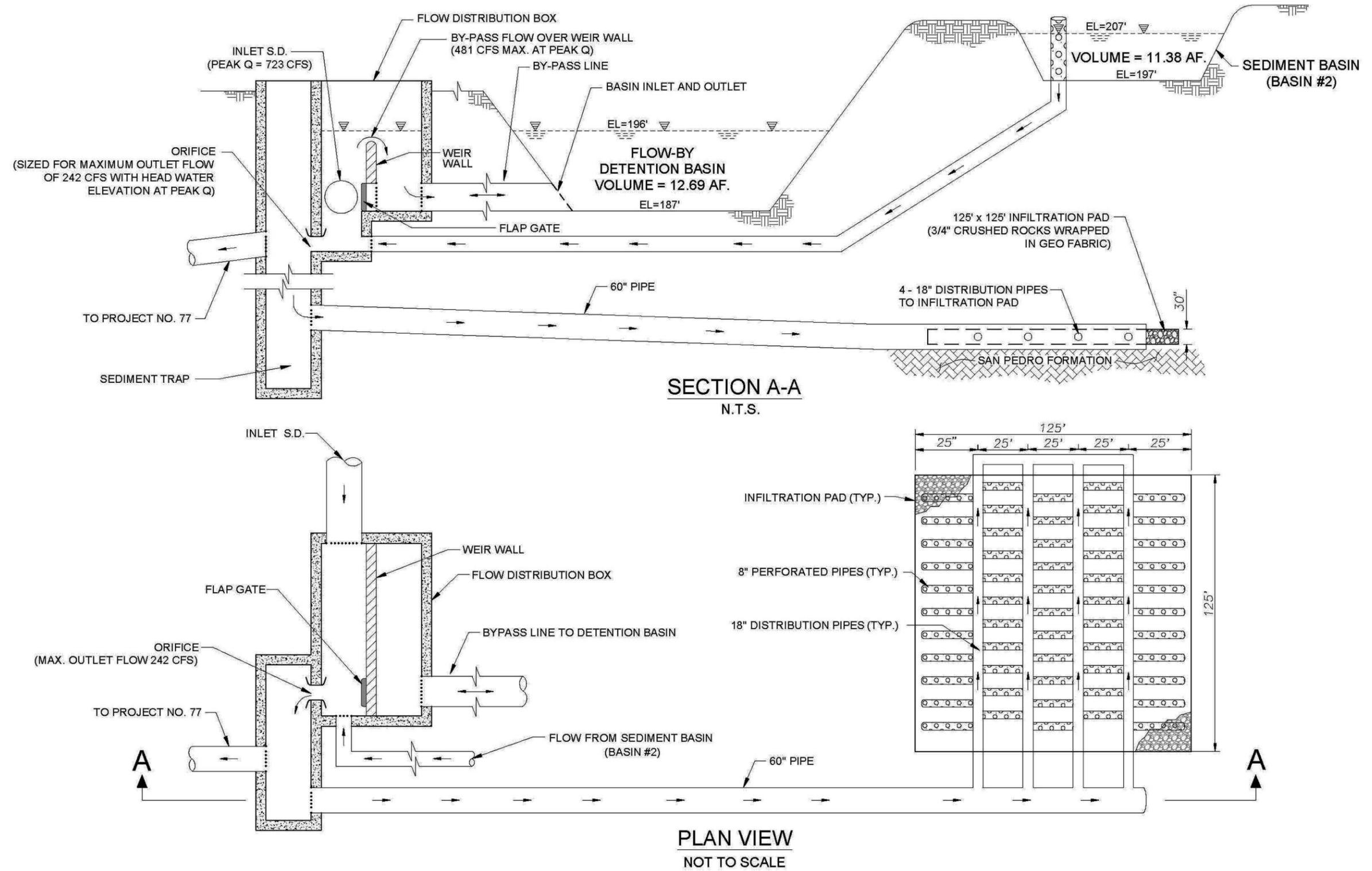
Figure 3-10: Chandler Quarry Project Infiltration System Concept Design
