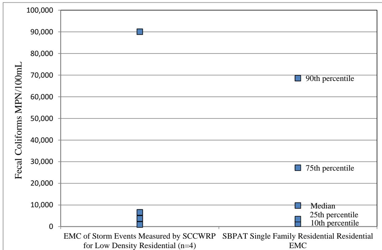
**Figure 7. Comparison of Fecal Coliform Low Density Residential EMC Values Between SCCWRP Measurements (n=4) and SBPAT Modeled Values (a full log distribution is used by the model, but non-parametric summary statistics are shown for comparison)**
