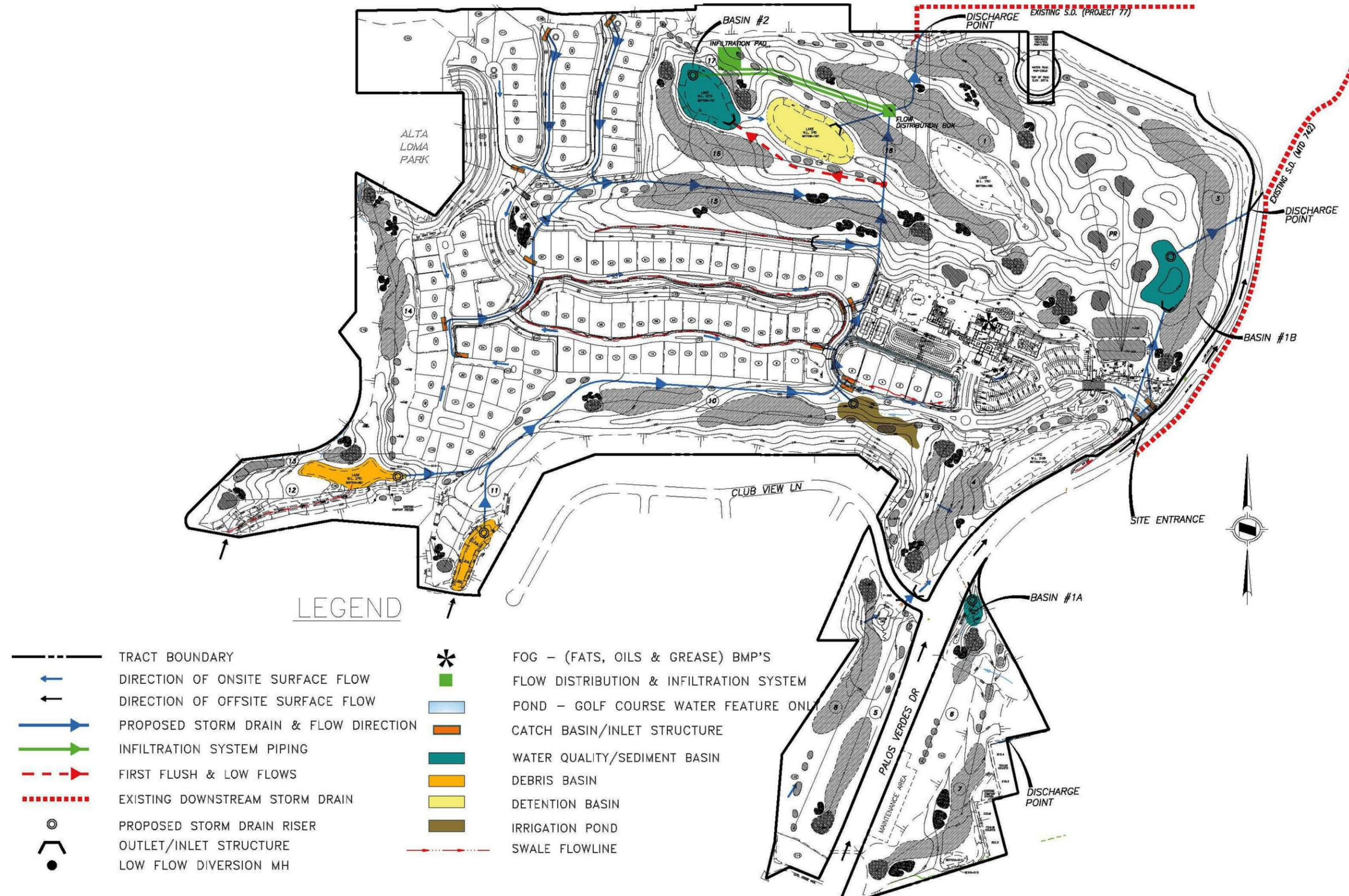
Figure 5: Chandler Quarry Project Drainage and Water Quality Concept Plan (Hunsaker and Associates. Water Quality Mitigation Plan. June 16, 2010).
