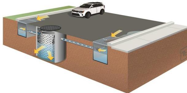
**Figure 3-5: Drywell schematic**
