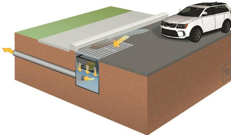
Figure 3-12: Pre-treatment BMP schematic
