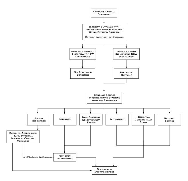
Figure 7. Non-Stormwater Outfall Screening Program
