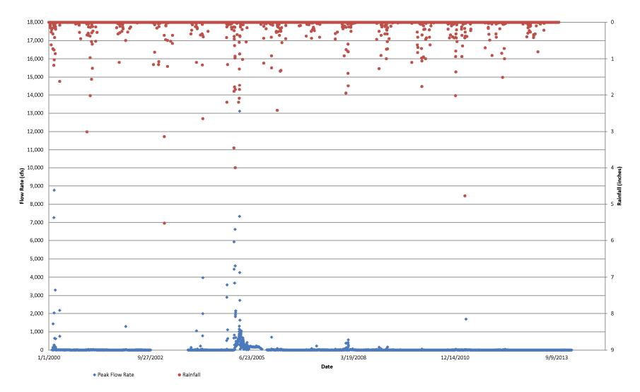
Figure 5. Peak Flow Rate and Rainfall Data for Santa Clara River Reach 5 at the Old Road Bridge<sup>8</sup>
