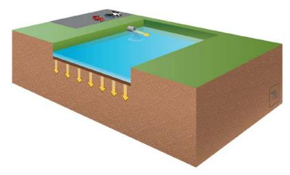
Figure 5-4. Conceptual schematic of regional BMP (arrows indicate water pathways)
