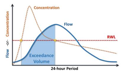
Figure 6-4. Illustration of How Metals Exceedance Volume is calculated for Critical Condition Determination
