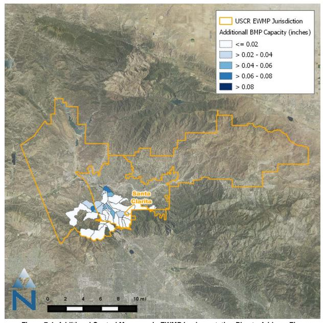
**Figure 7-4.** Additional Control Measures in EWMP Implementation Plan to Address Zinc This map uses the same approach as **Figure 7-3** to present the additional capacity in the EWMP Implementation Plan to address metals (beyond the control measures to address *E. coli*). Only subwatersheds within the South Fork assessment area require additional capacity beyond what was presented in the previous figure. The tabular version of this map is presented in Appendix D-1.
