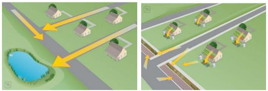
Figure 5-1. Conceptual Schematic of Regional (left) and Distributed (right) BMP Approaches
