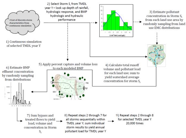
Figure 3-2 Structural BMP Prioritization and Analysis Tool Monte Carlo Methodology
