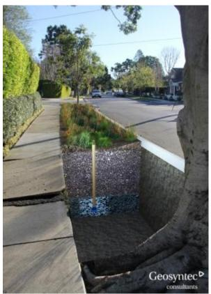
Figure 4-22 Section View of Bioretention with Underdrain
