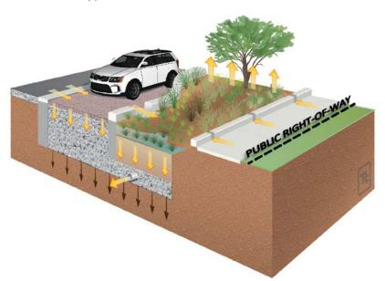
Figure 4-23 Typical Distributed Green Street Schematic
