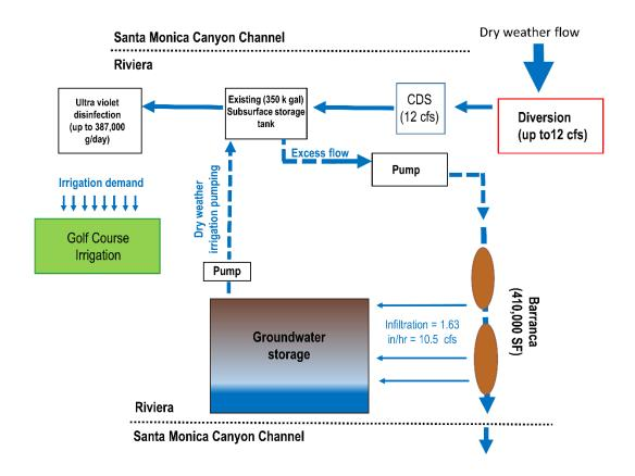
Figure 7. Alternative 1 (existing tank only) dry weather process flow diagram.
