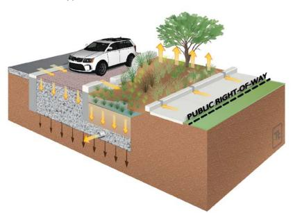
Figure 4-23 Typical Distributed Green Street Schematic
