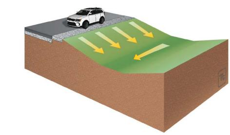
Figure 4-25 Typical Bioswale Schematic
