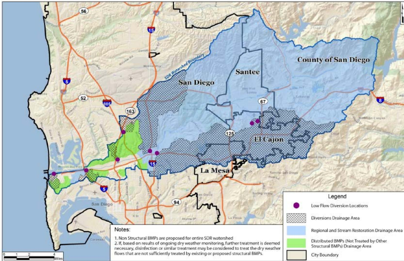
Figure 24. Dry weather flow area treated by proposed structural BMPs
