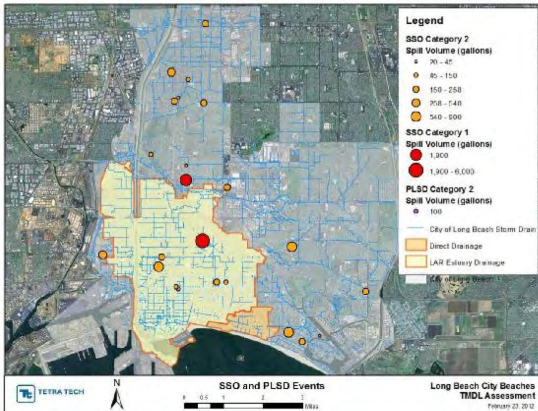
Figure 5-6. 2011 SSOs and PLSDs in the direct drainages
