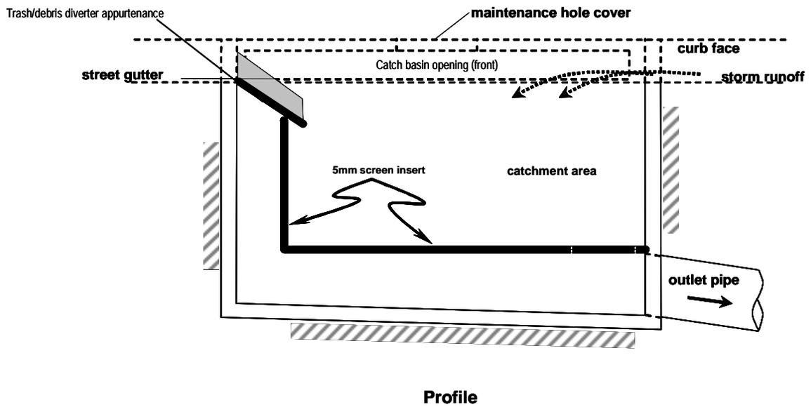
Figure 1.3 Typical Insert Installation
