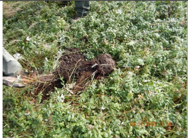
Photo 24: Area C. Inspector dug a hole in the lower elevation of the remnant slough channel, which showed a high concentration of river gravel.
