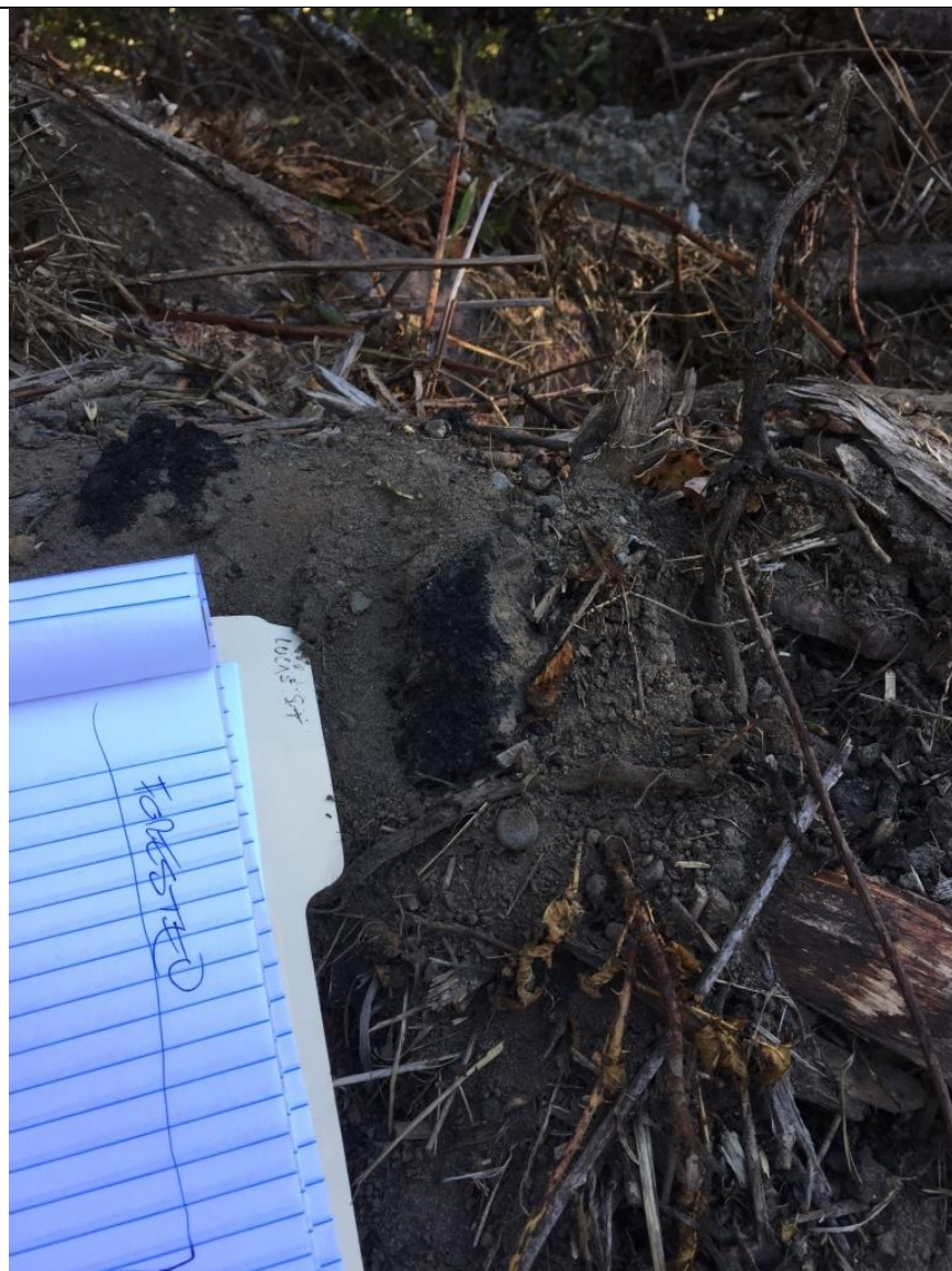
Figure 37: The debris pile consisted largely of woody vegetation and dirt, but debris such as asphalt, concrete, and brick was also within the debris pile. This photo shows two pieces of asphalt mixed in with the other debris.
