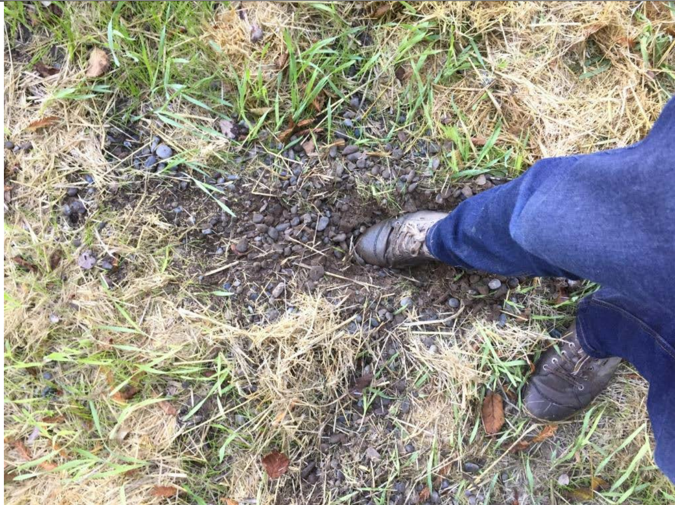
Figure 35: Light scraping of the soil with my shoe in the area represented by the orange line in Figure 34 uncovered a large concentration of rounded gravel. The presence of this rock suggested that it was backfill rather than native material, and the linear nature of the indentation suggests that there may be a pipe buried in this location. There may be an outfall for this pipe adjacent the Third Slough culvert in the area described in Figure 29.
