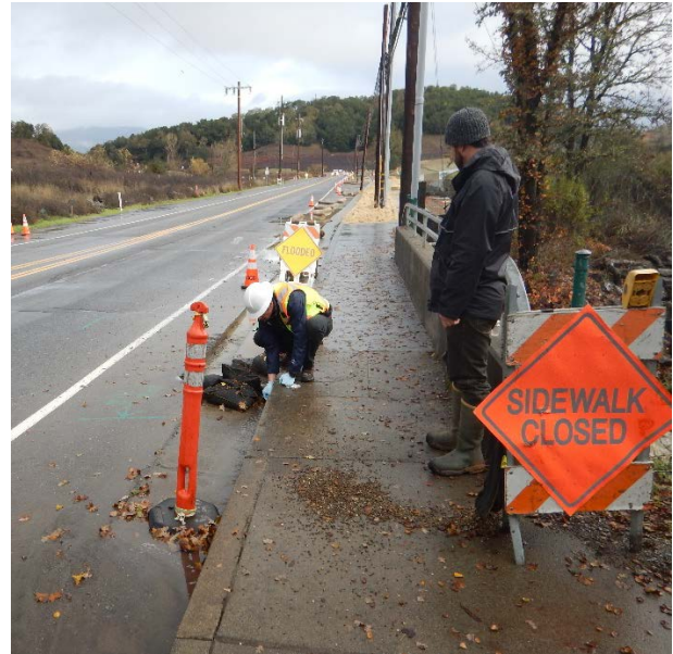
Pictures 2a and 2b above. Pic 2a (left) shows a turbid discharge from construction Site entrance along Healdsburg Avenue. Pic 2b shows Regional Water Board sampling the turbid storm water discharge from the project entrance (367 NTU). Additionally, a background storm water sample was collected from Healdsburg Ave (72.7 NTU).
