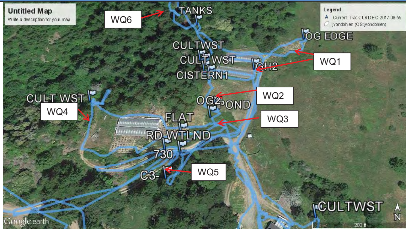
Figure 3. Inspection Map – Upper Property. Blue track identifies inspection route as recorded on Garmin GPS. Way points indicate features of interest with respect to water quality. WQ numbers (WQ-X) indicate a water quality violation or recommendation.
