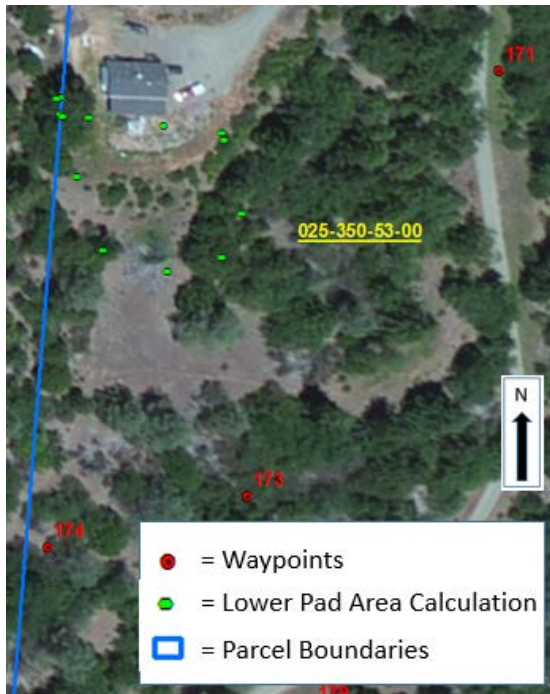
Figure 8: Green dots depict the perimeter of the expanded portion of the pad. WP-174 and WP-173 mark two locations along the toe of the pad.
