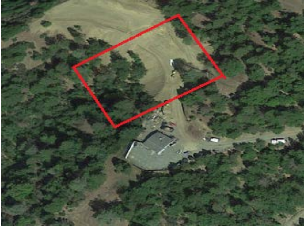
Figure 15: The red rectangle outlines the approximate area of surface drainage affected by filling in the watercourse. Notice how soil was side cast (discharged) in the upper reach of the canyon (Google Earth Pro, 2017).
