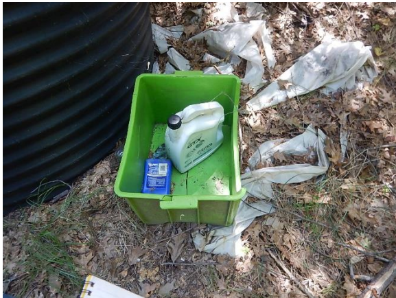
Figure 48. Oil is stored in a plastic tote; the plastic tote is cracked and would readily leak spilled material.
