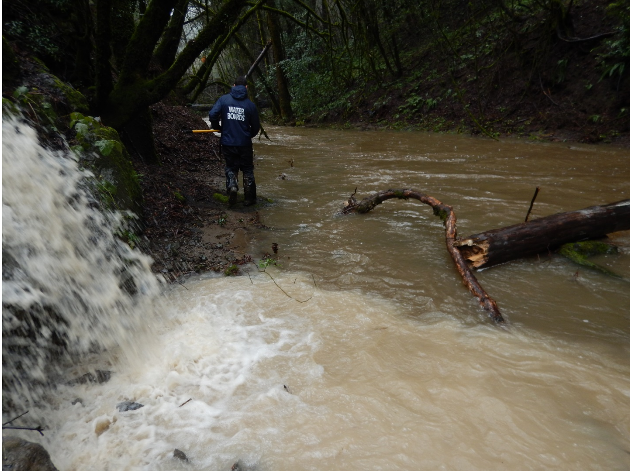
Photo 2: East culvert discharge to Porter Creek looking upstream. Elevated sediment content is evident in the discharging water and confirmed by the turbidity measurements. Photographed by Paul Nelson.
