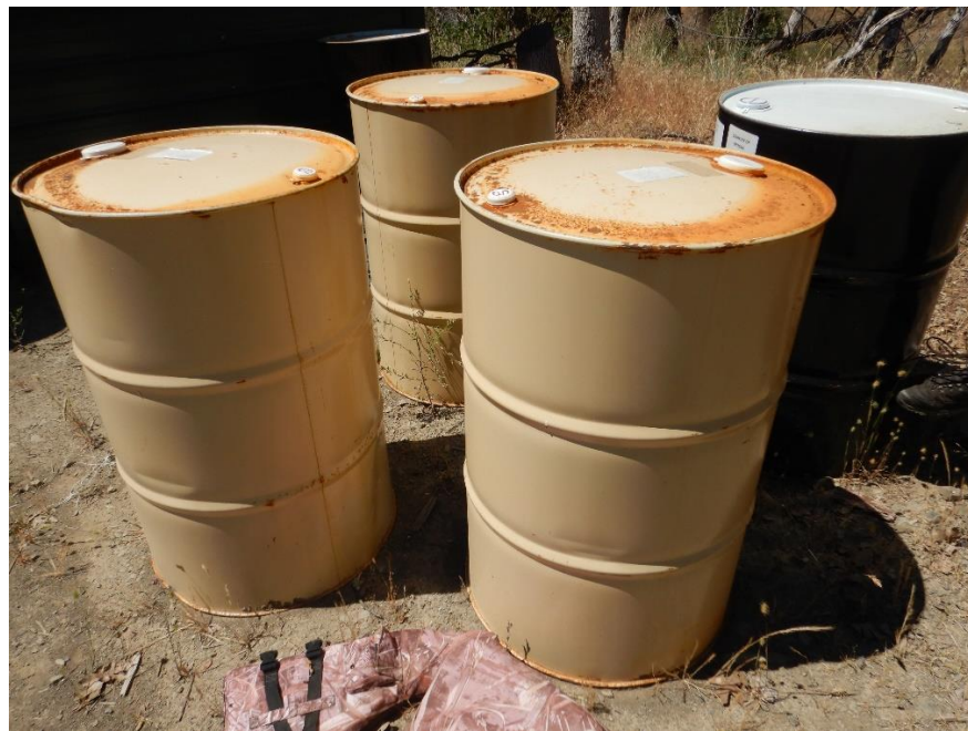
photo 14 —55-gallon drums of Gaco Western ISO-52 ISO component A, and 183M Polyol Component B, sitting on bare ground at WQ 12.
